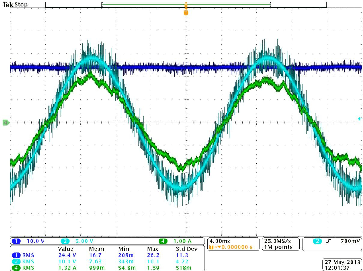
**Fig. 5: Active rectifier voltages and phase current under steady-state**
