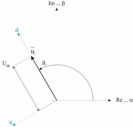
**Fig. 2: Definition of rotating d,q reference frame**
