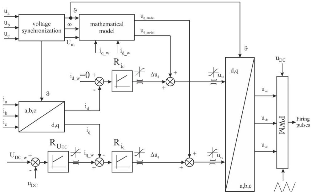
**Fig. 3: General structure of vector control for voltage source inverter**
