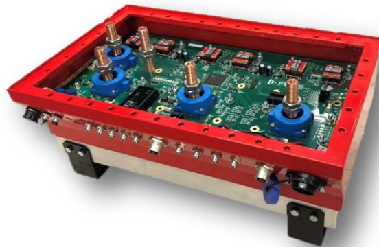
Figure 9. Control board with 3-phase inverter
