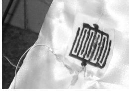
Figure 3. Example of interdigital capacitive sensor hand-painted on textile, identical with one used in [5].
