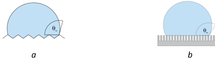
Fig. 2.1.1. Wetting of a textured surface. a – wetting of a low roughness surface; b – hydrophobicity on a surface with high density of textured microobjects [27].
