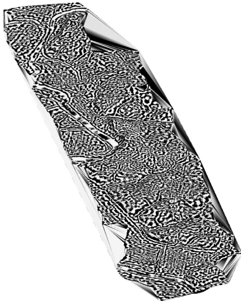
Fig. 7. The signed errors for the Serpent Mound dataset and Wendland's RBF \phi_{3,1} with \alpha = 0.01 : the positive error is colored white and the negative error is colored black.
