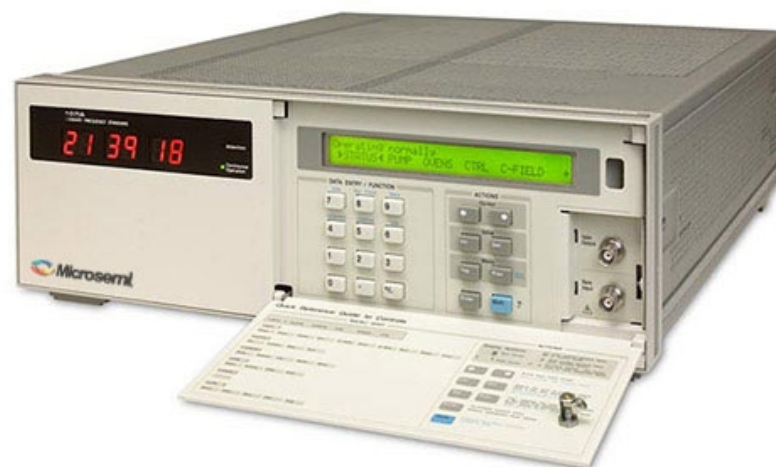
Figure 3.2: Microsemi brand Caesium standard
