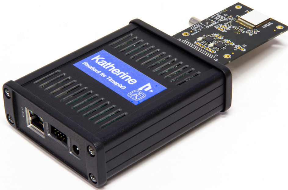
Figure 9.1: Katherine readout for Timepix3
