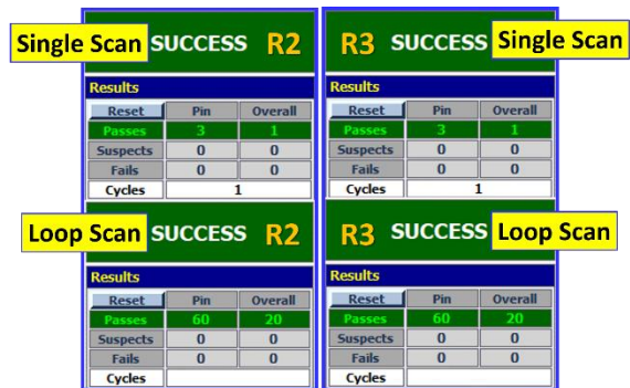
Fig. 18: Single scan mode and loop mode comparison for reference samples of the 4PP04L03 transistor
