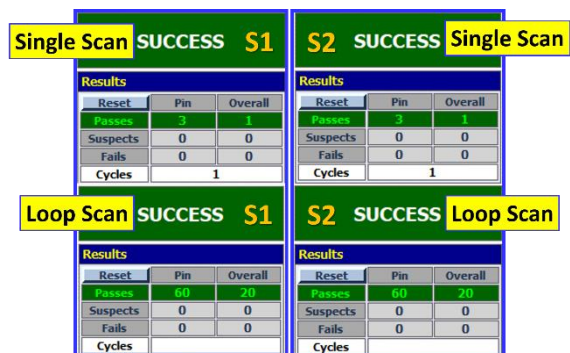
Fig. 19: Single scan mode and loop mode comparison for evaluated samples of the 4PP04L03 transistor.
