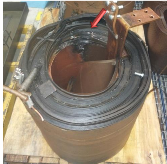
Fig. 9: LV coil foil winding. The short occurred at the top of the LV coil about 80 degrees to the right of the LV busbar. The destruction leads from the first layer of Cu conductors to the ninth. (It is possible that a developing fault in the HV winding has affected this adjacent LV winding.)
