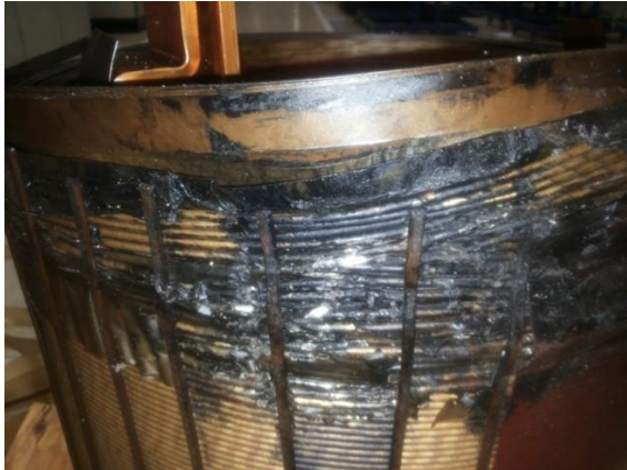
Fig. 7: Exposed damaged winding of the transformer HV coil. The short circuit is located about 50 degrees from the busbar. The combustion plant has an irregular shape and a range from the surface to the first cooling channel.
