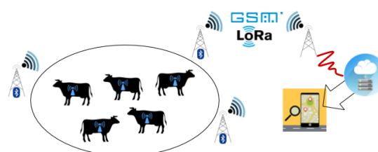
Figure 1: Principle of the e-Cattle system
