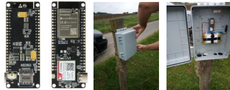
Figure 4: a) ESP32 T-Call modul for Hub, b) installation box c) internals of Hub
