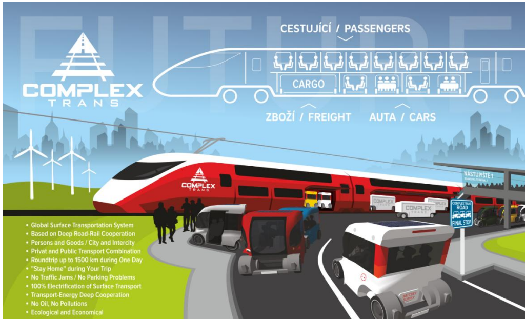
FIG.1 - platform of the ComplexTrans system: passengers change (upper deck) and loading and disloading of adapted cars (coupemobiles) with passengers and freight modules (lower deck) in the ComplexTrans trains.
