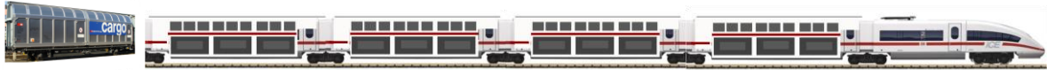
FIG. 2 - individual fast freight wagons or their small groups are connected and disconnected to/from the back of ComplexTrans trains with double-deck passengers-freight coaches.
