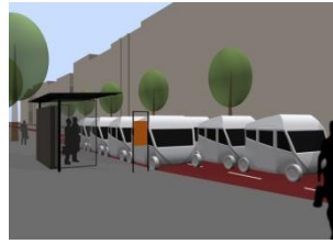
FIG.20 – a platoon of coupemobiles is formed at the stop, another platoon is just passing by.
