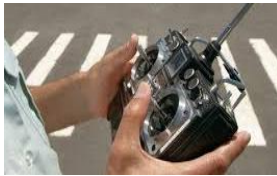
FIG.22 – the remote control is used for local handling of the freight transport module.
