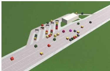
FIG.17 – coupemobiles can also be coupled mechanically using a coupler placed on the extendable axles. For coupling of the coupemobiles with the same direction will be used sorting terminals.
