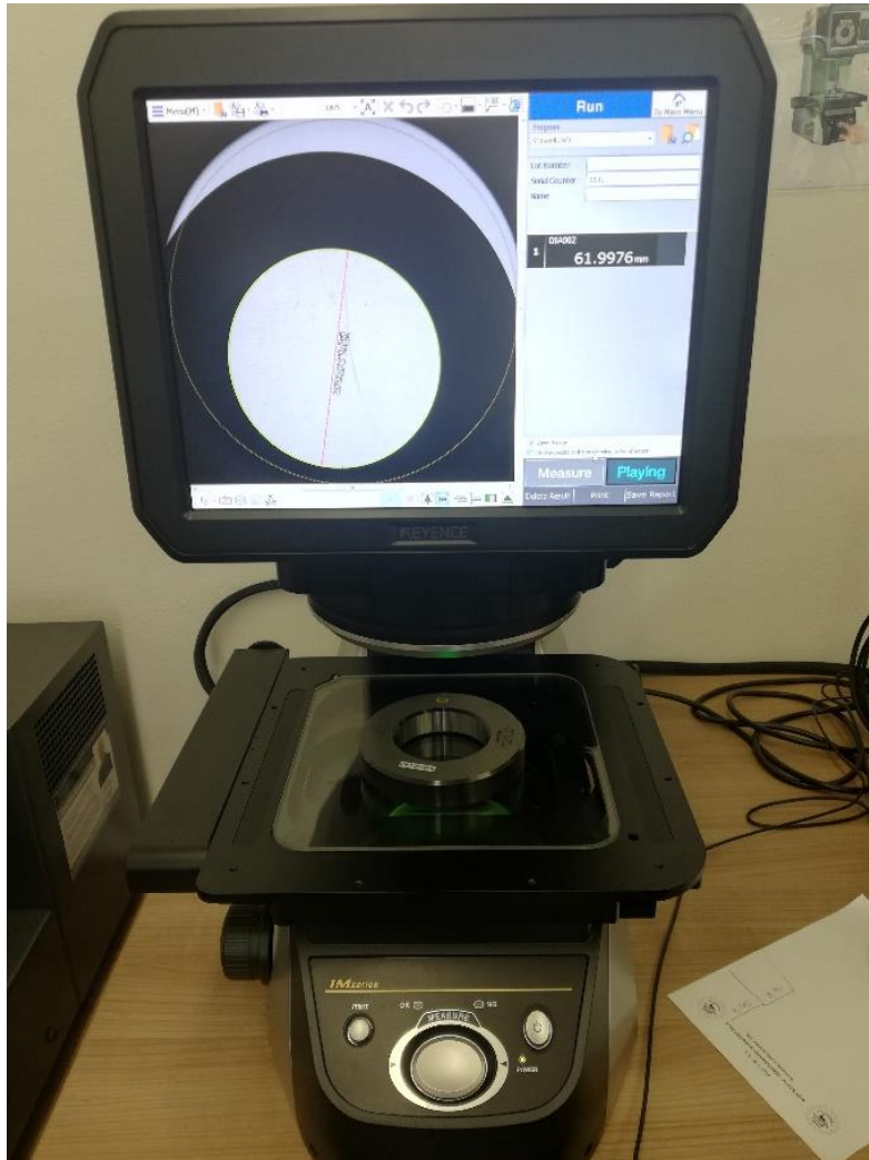
Fig. 1. Optical comparator Keyence IM-7000
