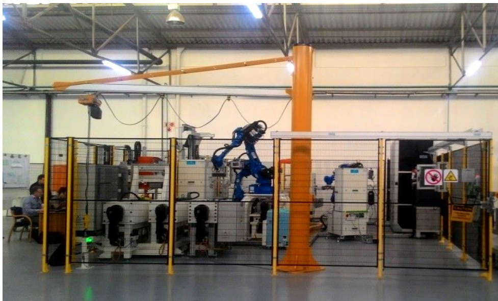
Fig. 2. Robotic inspection line
