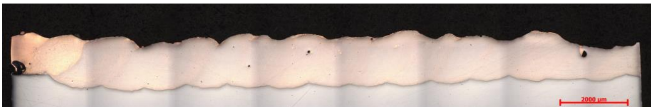
Fig. 2. SAMPLE A - Macrograph of a transverse section through the laser overlay; unetched; magnification 25×
