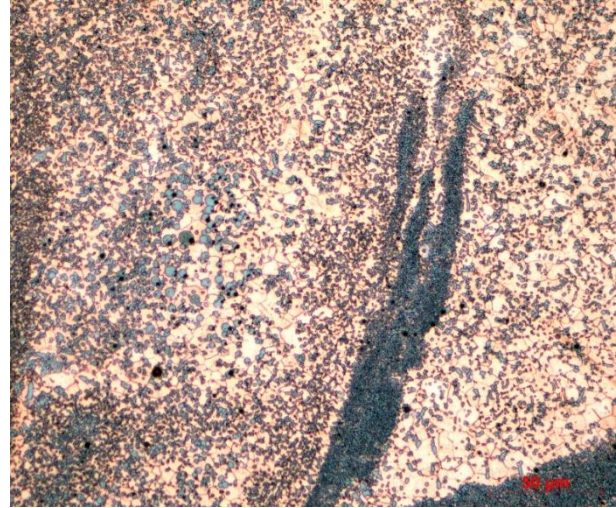
Fig. 4. SAMPLE C – Metallographic structure of the transition region between two beads; etched with Robin's reagent; magnification 500 \times [11]
