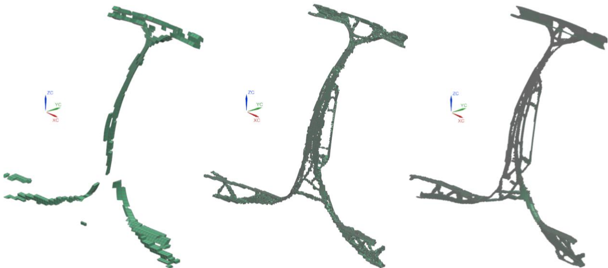
Figure 3. Results with HEXA 8- size 20mm (left), hybrid mesh – size 10mm (middle), HEXA 8- size 5mm (right)
