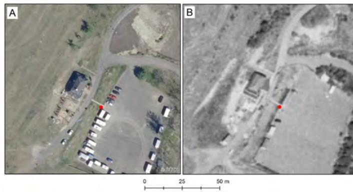
*Figure 3 Example of Ground Control Point identification. A – contemporary orthophoto available as WMS. B – processed orthophoto from 2008.*
