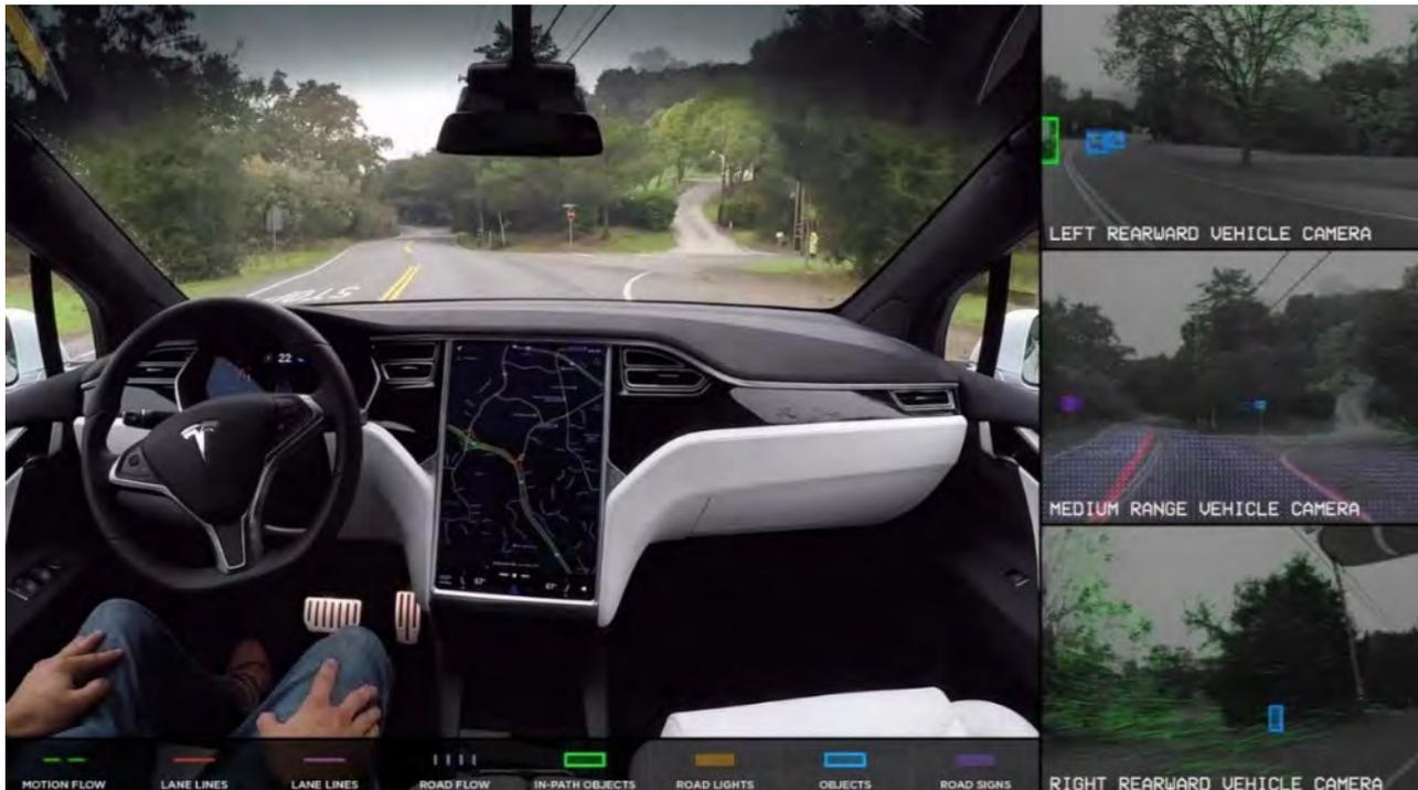
Figure 1. The interior of a driverless car and the road objects detected by the cameras (The Tesla Team 2016)
