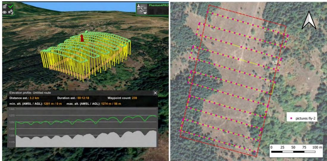
Figure 4. Flight mission FP2: (a) UgCS work screen ; (b) Location of the taken images
