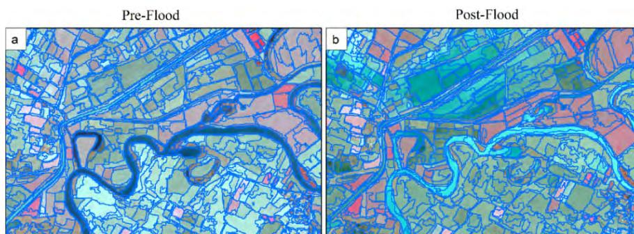
Figure 3. Image segmentation results of sample region for (a) pre-flood and (b) post-flood Sentinel-2 MSI images.
