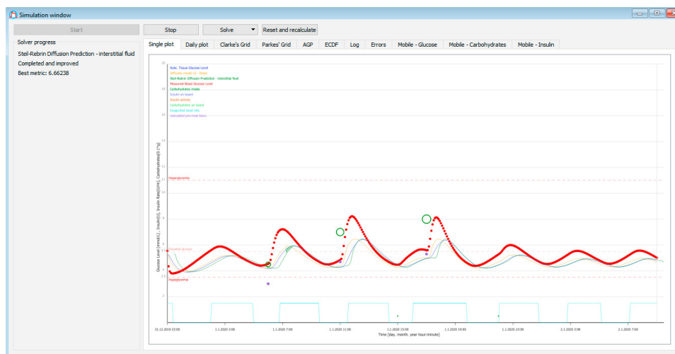
Fig. 5. Visualization of Predictive Low-Glucose Management system built with SmartCGMS.
