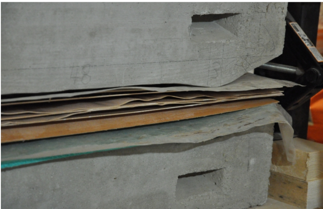
I always put a sheet of camping mat under the wood layers. It smooths any imperfection of the concrete mold.
