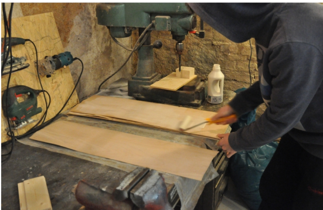
For coating the sheets with glue I am using a foam paint roller. On one deck 0,5 l of glue is spent. I coat every layer (except from the face veneers) from both sides.
