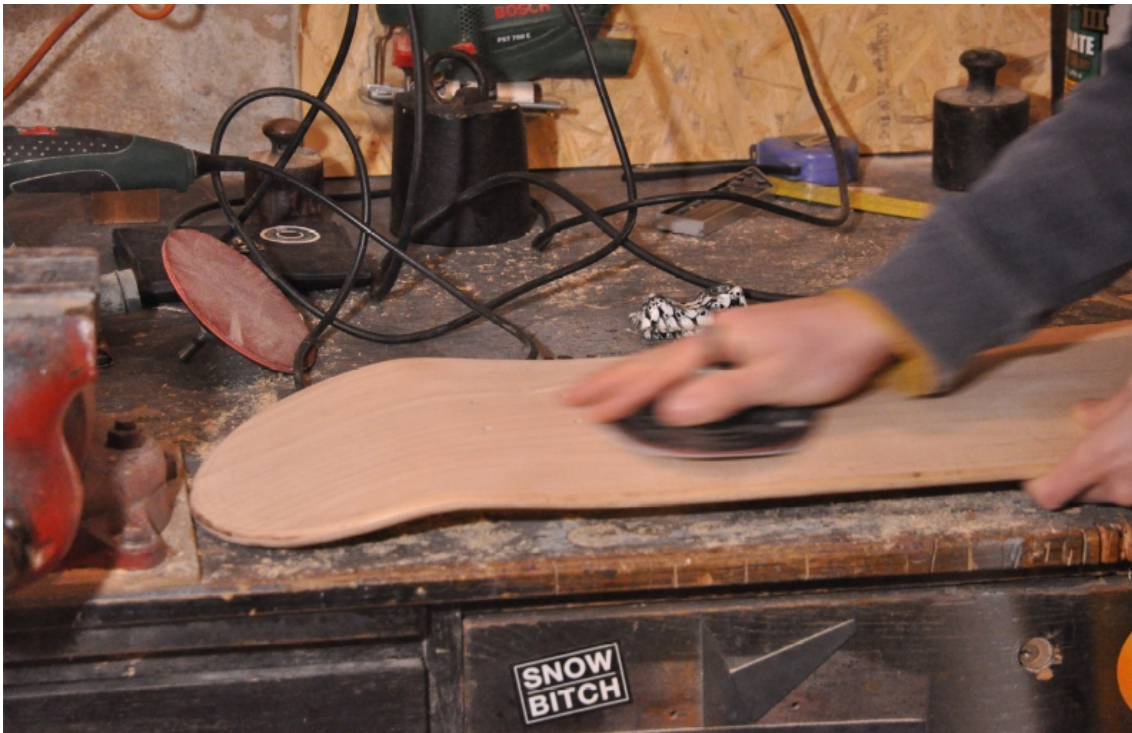
smoothing remaining imperfections
