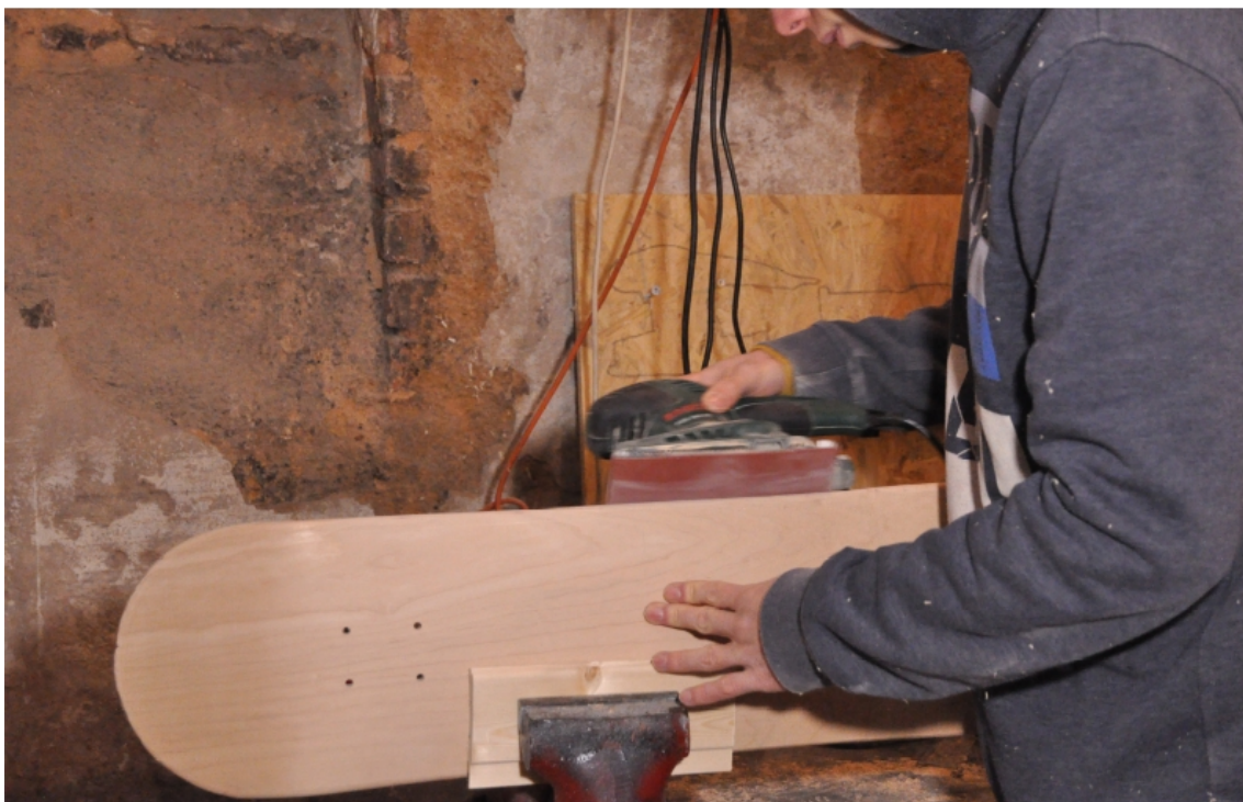
One of the last steps is sanding which creates a smooth surface. A vibrating or an orbital sander is the best performing machine.
