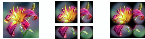
(b) Vignette operation (with a radial size of 0.58 and a radial smoothness of 0.21) applied to one level of a DZI without UV correction.
