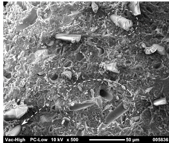
Figure 7. SEM image of hardened paste with 20 wt% of basalt fibers.
