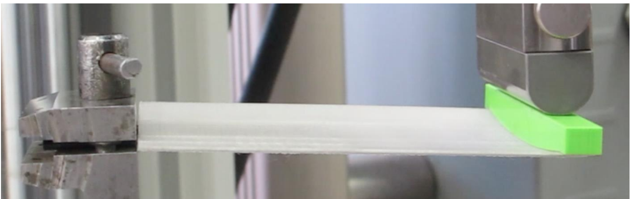
Fig. 5. Test of bending stiffness
