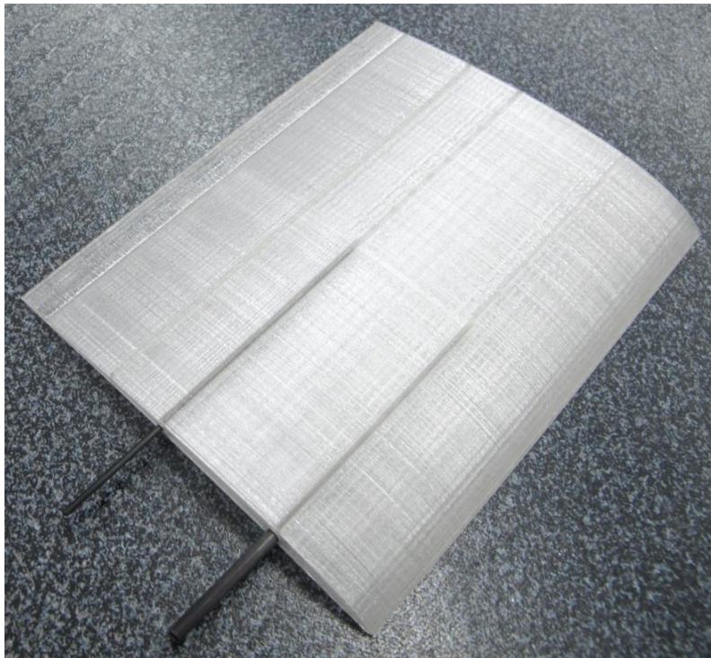
Fig. 7. The finished first part of the wing
