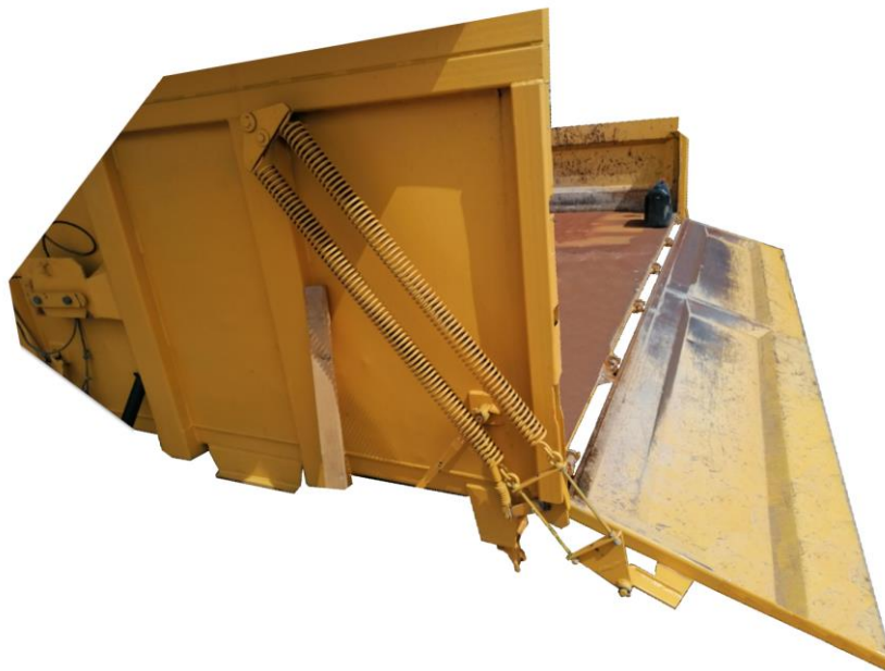
Fig. 1. Tipper body with spring mechanism, opened sidewall
