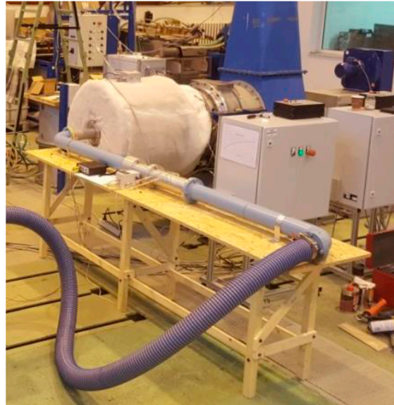
Figure 7. Extension of the VT-400 test rig with tip leakage calibration device [12].
