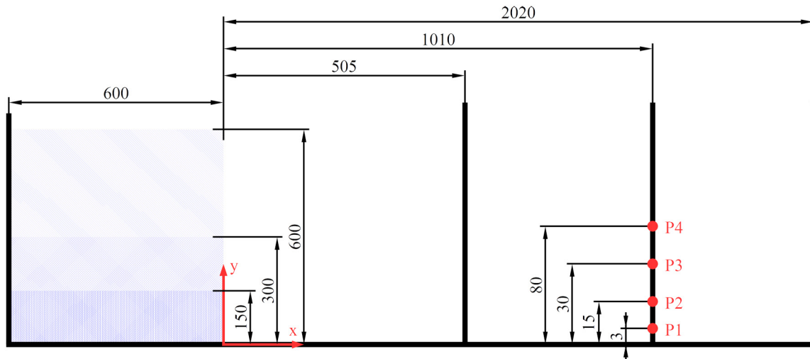
Fig. 1. Scheme of the problem with highlighted pressure probes for validation purposes. All dimensions are in millimeters
