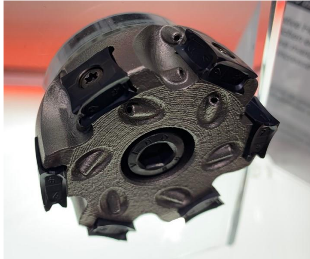
Fig. 2. A tool developed using 3D printing and optimization of cooling channels [5]
