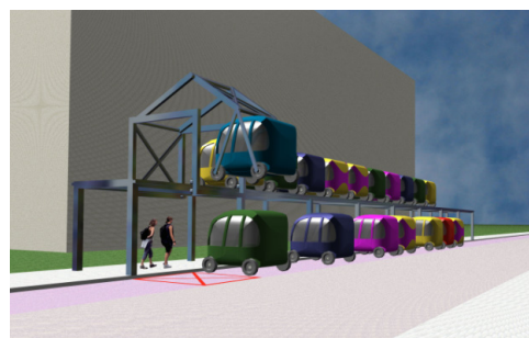
Fig. 13 Thanks to its compact shape and roof catch points, coupe-mobiles can be parked in special parking facilities above the sidewalks.
