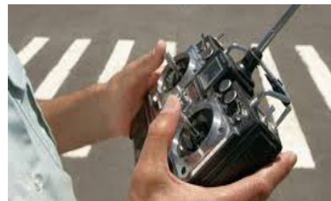
Fig. 22 The remote control is used for local handling of the freight transport module.
