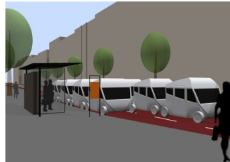
Fig. 20 A platoon of coupe-mobiles is formed at the stop, another platoon is just passing by.
