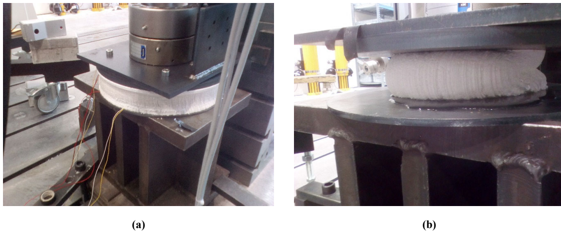
Figure 4-5: Deformation and failure mechanisms: (a) Regular sample deformation occurring for lower H/D, (b) Buckling-form deformation occurring at larger H/D
