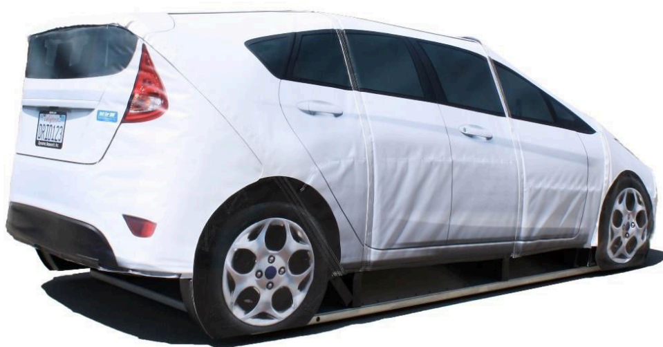
Fig. 3.6: Example of the Global Vehicle Target (GVT) |Borrowed from [17]|
