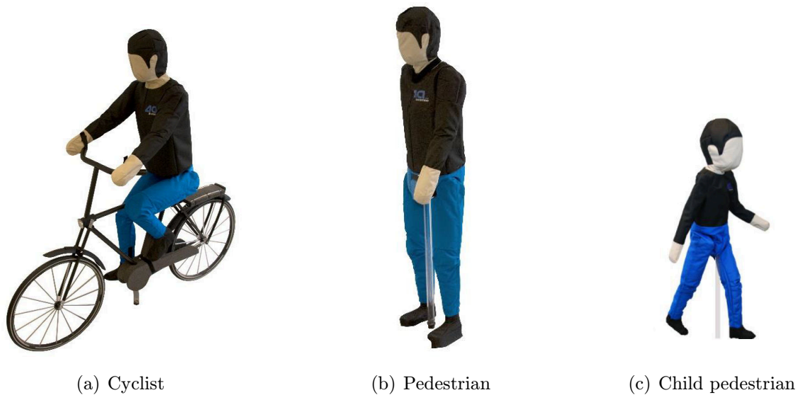
Fig. 3.5: Examples of the Euro NCAP targets |Borrowed from [17]|
