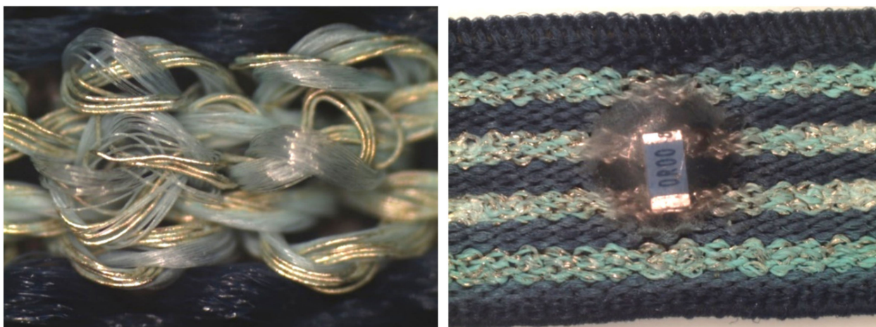
Figure 10. Details of the sample after aging by artificial sweat.
