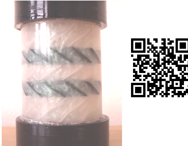
Figure 5: Axial compressor in a transparent plexiglass tube moved by hand. The QR-code links to a movie: https://youtu.be/DHj101R265M . Special thanks to Michaela Vacková for the plexiglass tube.
