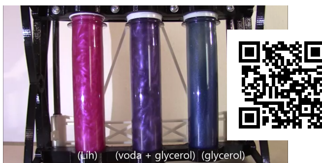
Figure 4: Three test tubes filled with different liquids, left ethanol, middle water + glycerin, right pure glycerin. All the tubes contain the same iron ball which is moved by a magnet which is on the white support in behind. The QR-code links to a movie: https://youtu.be/dxcRUnd9Bp8 . Special thanks to Ing. Martin Pelikán for the set of iron balls of same dimensions and to Michaela Vacková for the set of PET tubes usually used as precursors of PET bottles.
