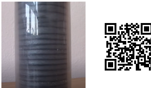
Figure 3: Taylor-Couette flow in a cylindrical cell with rotating inner cylinder. The QR-code links to a movie: https://youtu.be/hbwH0uvp2nE .
