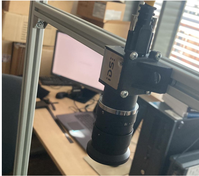
Figure 4.3: Aluminium profile frame with mounted camera
