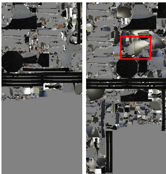
Figure 5. Atlas of patches generated for Chess sequence: depth-dependent pruning (left) vs. proposal (right).
