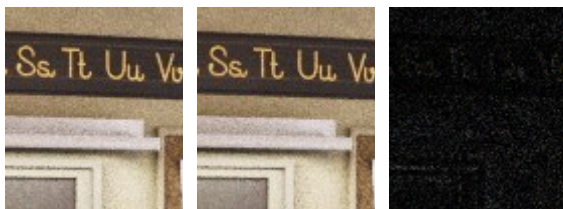
Figure 6. Fragments of two consecutive frames of ClassroomVideo sequence and the difference between them (on the right).
