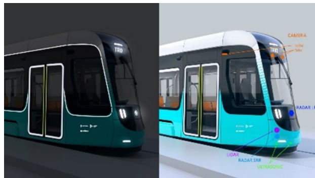
Figure 6: Skoda Transportation safe front end, source Project Final Report [4]
