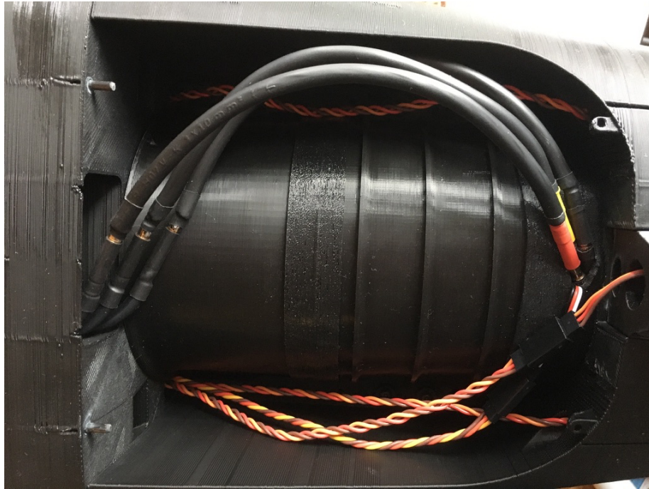
Figure 6: EDF assembly installed inside of the fuselage
