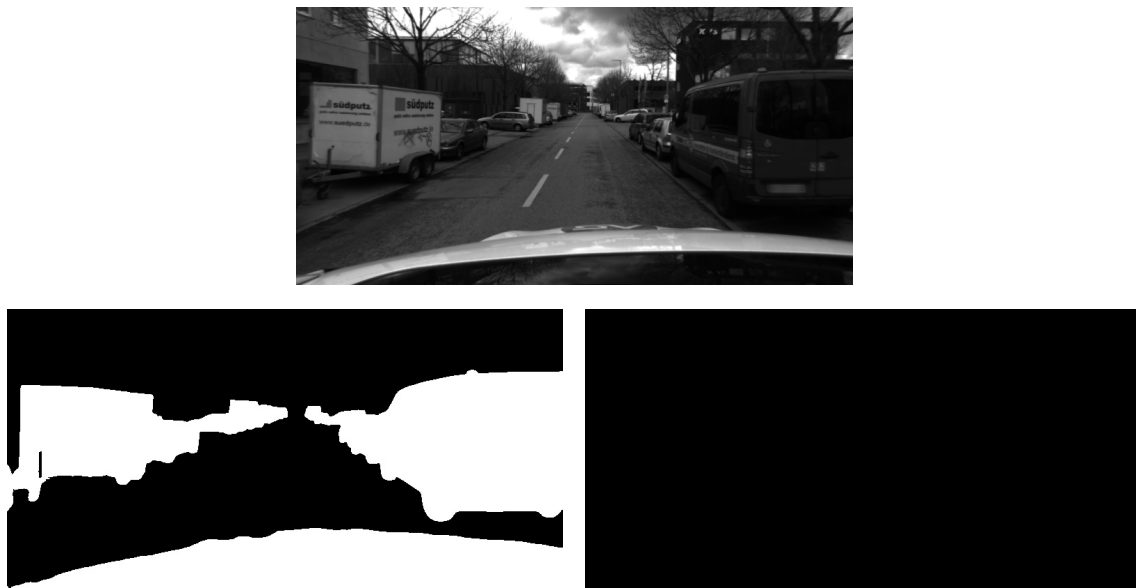
Figure 10.1: Top: an example from 4Seasons dataset. Left: binary mask for vehicle group of classes. Right: binary mask for human group of classes (it is empty because no human is presented in the image).
