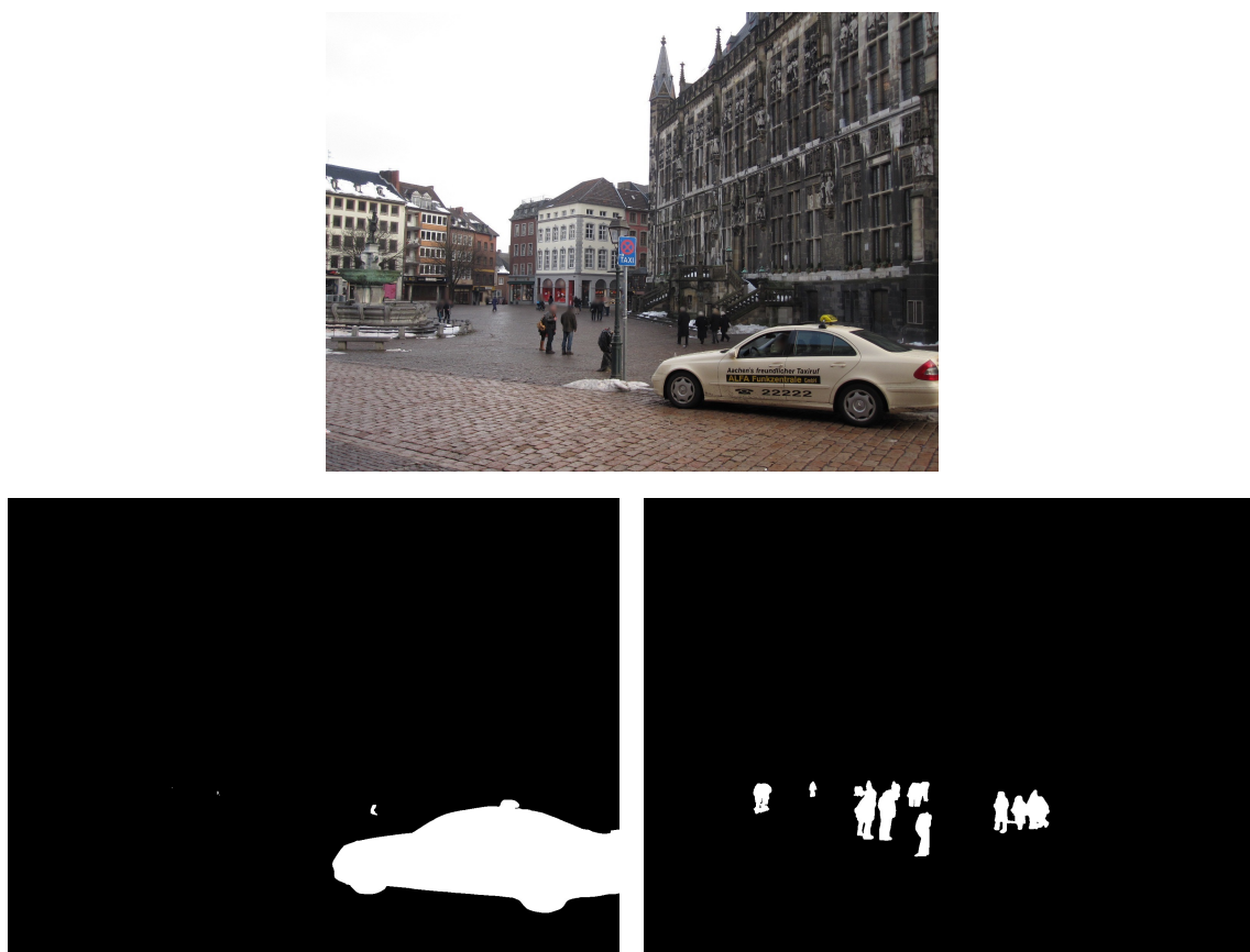
Figure 10.2: Top: an example from Aachen dataset. Left: binary mask for vehicle group of classes. Right: binary mask for human group of classes.
