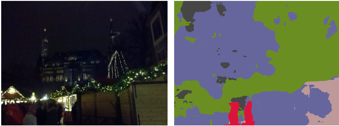
Figure 8.1: Left: original image from Aachen Night dataset. Right: failed semantic segmentation where the people (red) in the left bottom corner are missing, vegetation (green) is poorly segmented specifically in the top right corner, and a wall (purple) is in the top left corner where the sky should be segmented instead.
