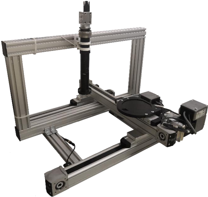
Fig. 3: Mechanical design of the WaferScan system, the final frame concept based on aluminum profiles and industrial stepper motors.
