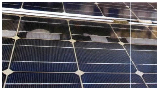
Fig. 6. Example of a delamination (Pilsen, CR, 2018 - 2021).
