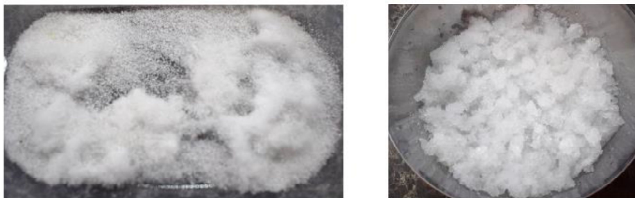
Figure 4. Demonstration of hydrogel from the diaper in the dry state and after soaking
