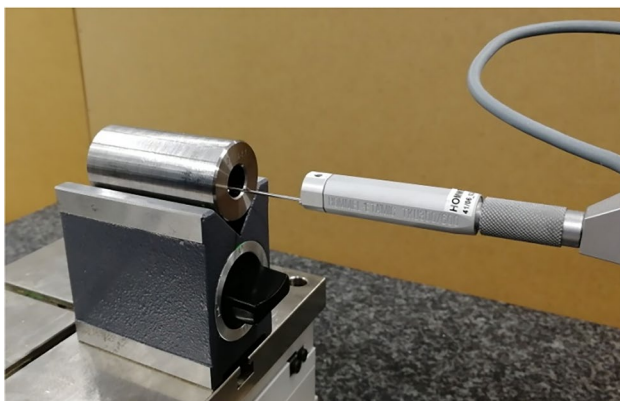
Fig. 6 Clamped specimen measured with Homel Etamic T8000 profilometer
