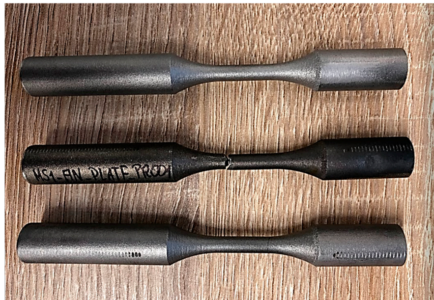
Figure 4. Photograph of test specimens before and after axial fatigue testing, OUtch Opole.
