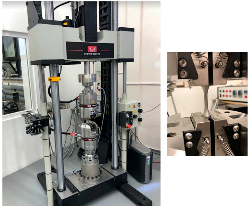
Figure 3. Fatigue test stand for tension–compression axial loading, Instron 8852, at Opole University of Technology.
