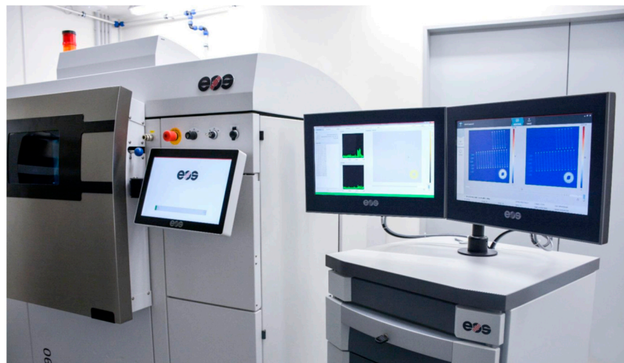
Figure 2. Selective laser sintering 3D printing machine EOS M290 used in the process of specimen preparation.
