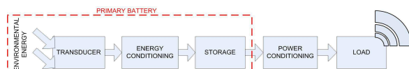
Fig.1 Block diagram of an autonomous system. The blocks inside the dashed red box form the energy harvester subsystem [1]
