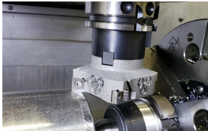
Fig. 3. Test machining of special tool with IC20 insert
