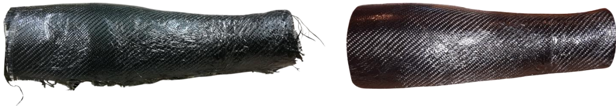
Fig. 6. Left - Raw product with sharp edges, right – final product round shape
