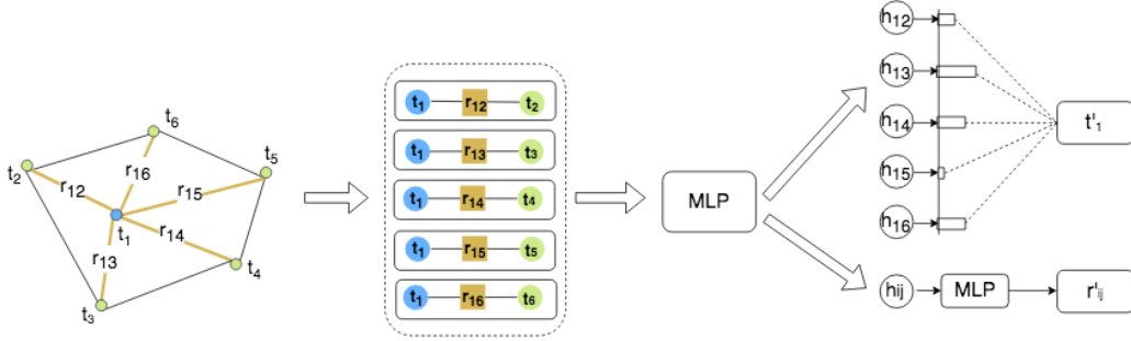
Figure 3.5: Contextualization of vertex ( t_i ) and edge ( r_i ) embeddings using a convolution operation - in this case, a multi-layer perceptron [42].
