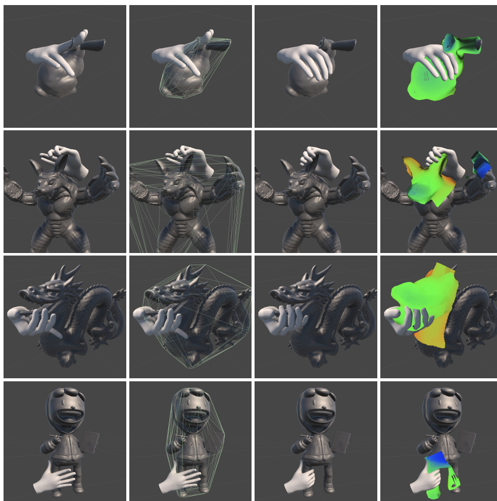
Figure 4: Example grasps of test objects including Stanford Bunny, Stanford Dragon, Stanford Armadillo, and Pixel mascot presented in four configurations: physics-based grasp, convex collider used for physics-based grasp, SDF sampling based grasp and SDF visualization
