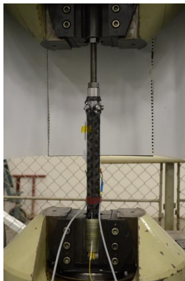
Fig. 2. Testing setup for composite tube with the DFOS sensor and strain gauges installed in axial configuration.
