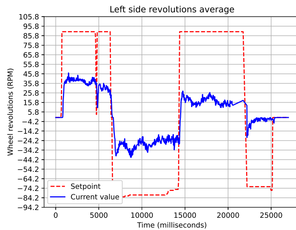
Figure 5.21: Average of \omega_1 and \omega_2 : \omega_L = \frac{\omega_1 + \omega_2}{2}
