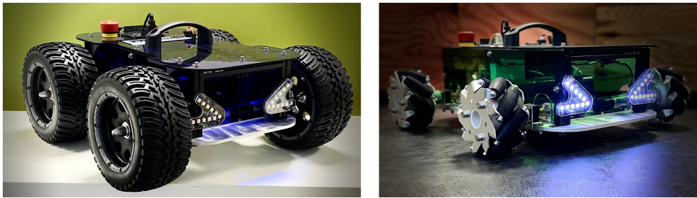
Figure 4.1: IoT Bot - differential drive variant (on the left) and mecanum drive variant (on the right) [12]
