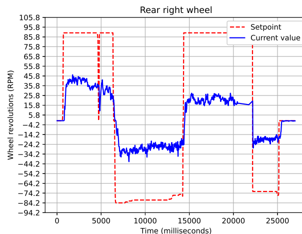
Figure 5.15: IOT Bot's rear right wheel's revolutions (setpoint \omega_4^* and actual value \omega_4 )
