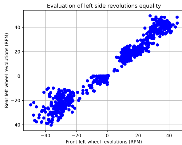
Figure 5.19: Evaluation of \omega_1 = \omega_2 (see equation 5.3) - using the actual values
