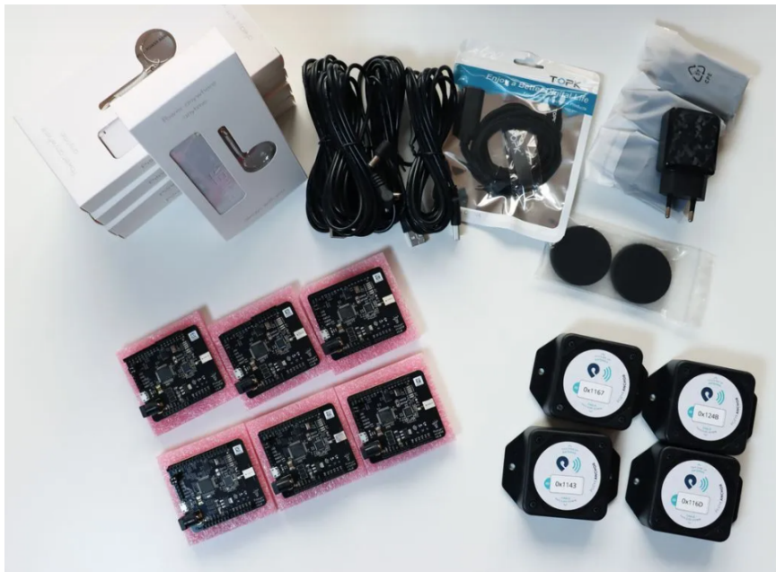
Figure 5.35: Pozyx creator kit (development tags on the left, boxes with static anchors on the right and wiring on top) [20]
