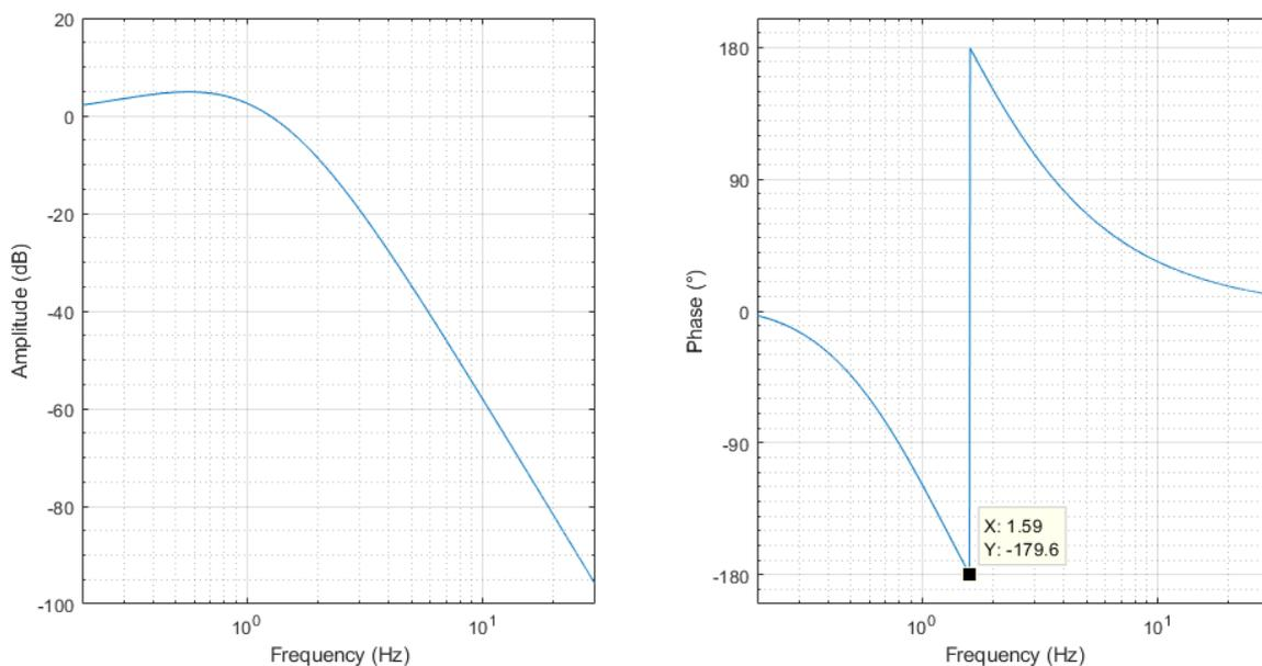
Figure 51 Torsional filter
