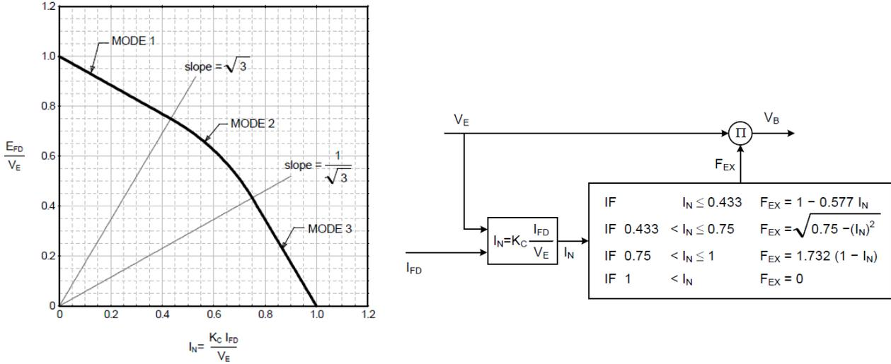
Figure 27 Function respecting the voltage drop at the rectifier ( $F_{EX}$ ) [8]
