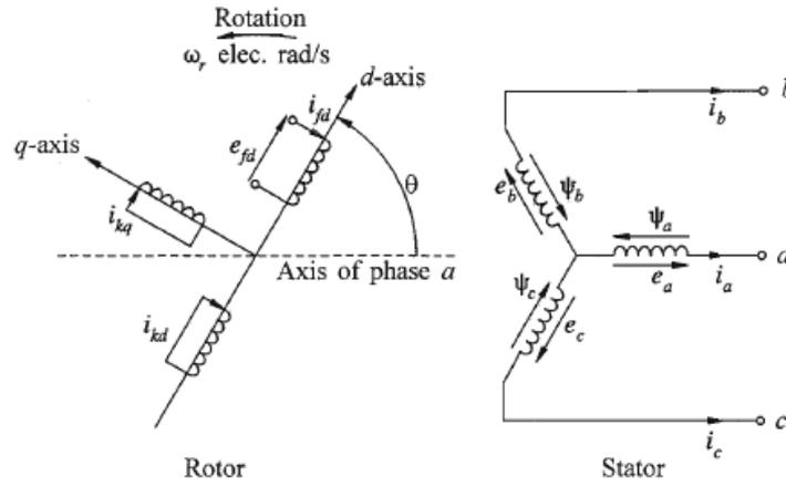
Figure 5 Synchronous machine windings and coordinate system [3]
