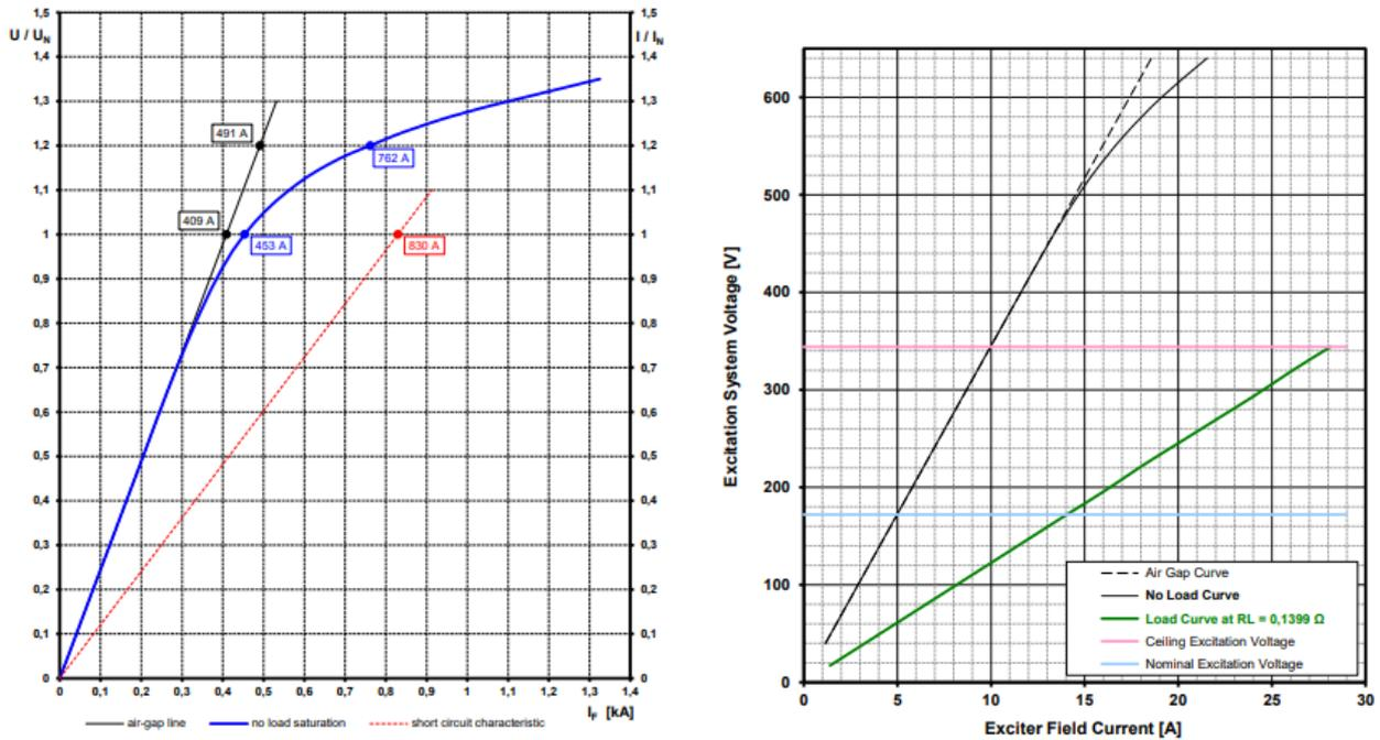
Figure 28 a) Generator characteristic, b) Exciter characteristic
