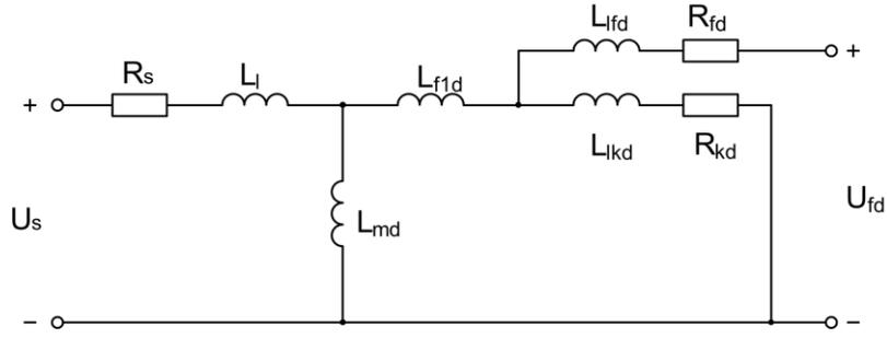
Figure 6 d-axis equivalent diagram
