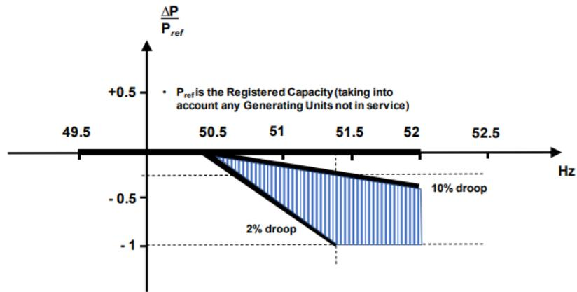
Figure 36 Active power frequency response of LFSM [1]
