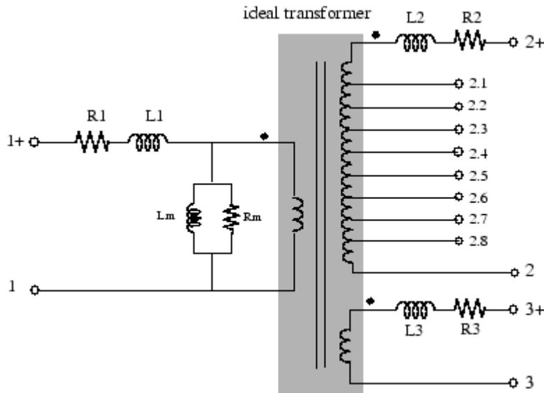
Figure 41 Equivalent circuit diagram of Multi-winding transformer [11]
