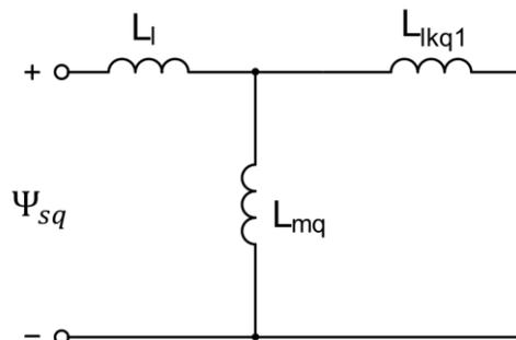
Figure 17 Equivalent circuit for \$L\_{q'}\$
