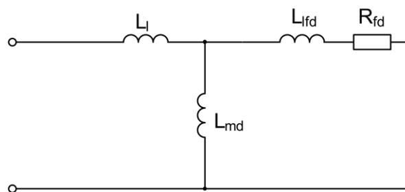
Figure 23 Simplified open-circuited diagram for the sub-transient interval ( $T_{d0}'$ )
