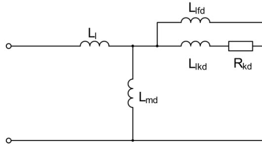
Figure 21 Simplified open-circuited diagram for the sub-transient interval ( $T_d''$ )
