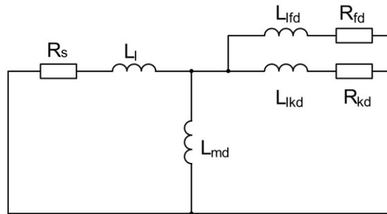
Figure 19 General short-circuited diagram for the sub-transient interval
