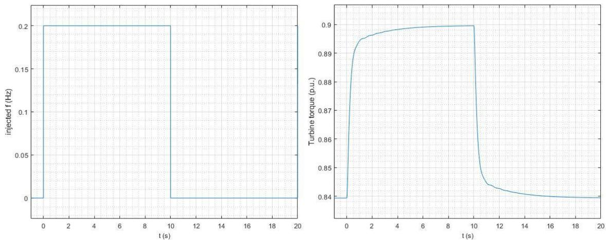
Figure 74 Turbine torque response to speed step
