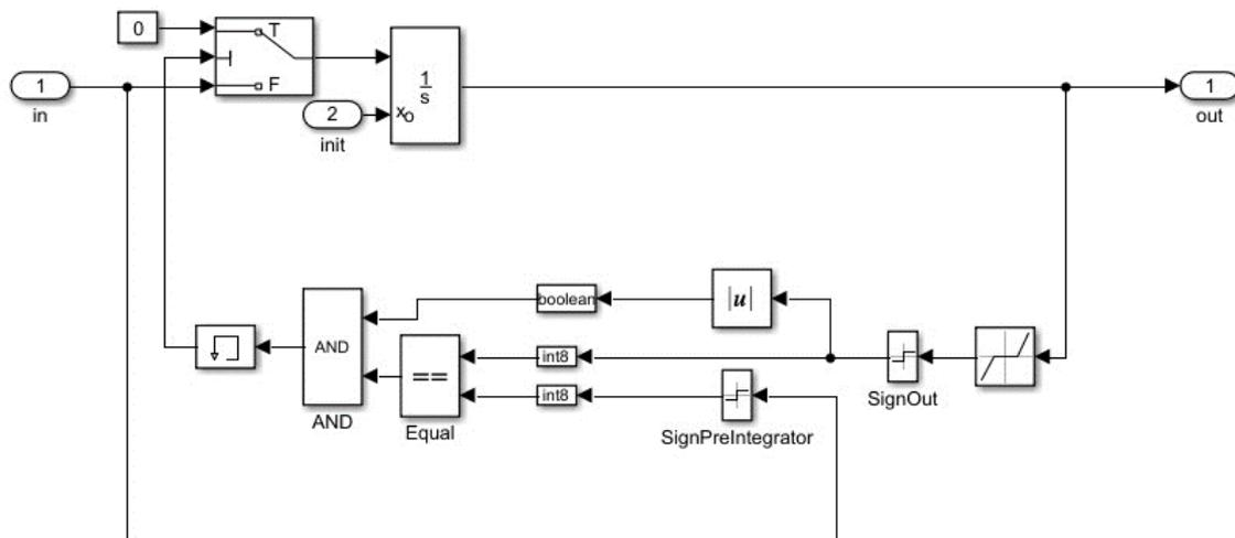
Figure 4 Anti-Windup of integrator
