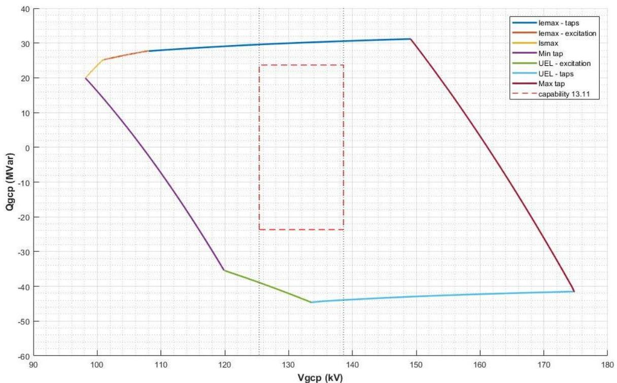
Figure 62 UQ capability diagram
