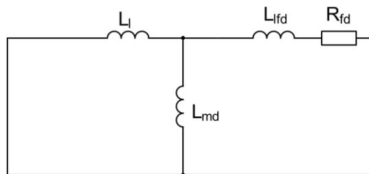
Figure 22 Simplified short-circuited diagram for the transient interval ( $T_d'$ )
