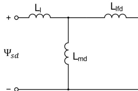
Figure 14 Equivalent circuit for  $L_d'$
