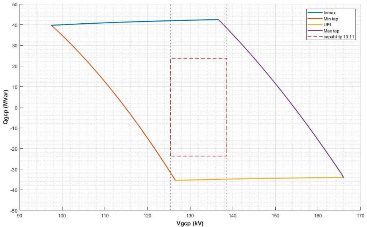
Figure 64 UQ capability diagram complying with specified conditions (iii) and (iv)
