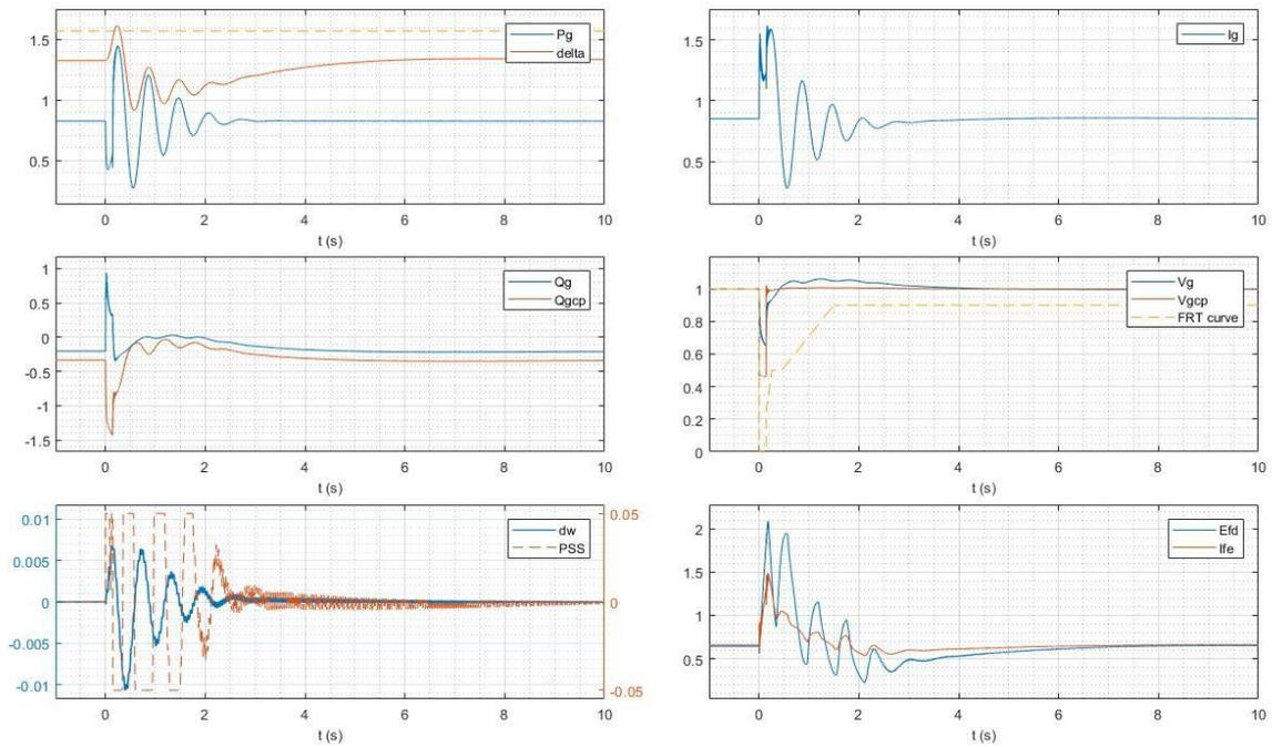
Figure 66 2-Ph to ground short circuit at transformer terminals for 140 ms
