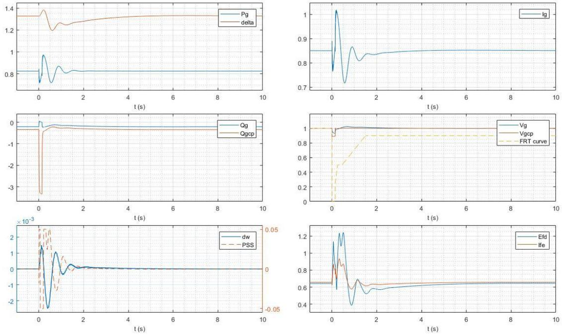
Figure 67 1-Ph to ground short circuit at transformer terminals for 140 ms
