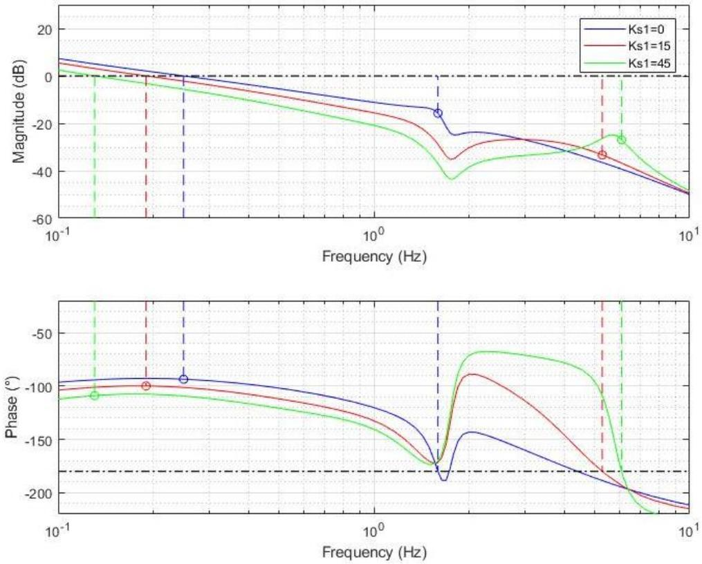
Figure 58 Bode plot  $V_g/V_{ref}$  in open loop
