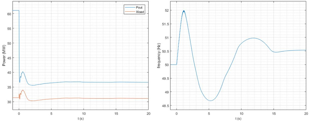
Figure 69 Grid cut-off with minimum possible connected load, LFSM
