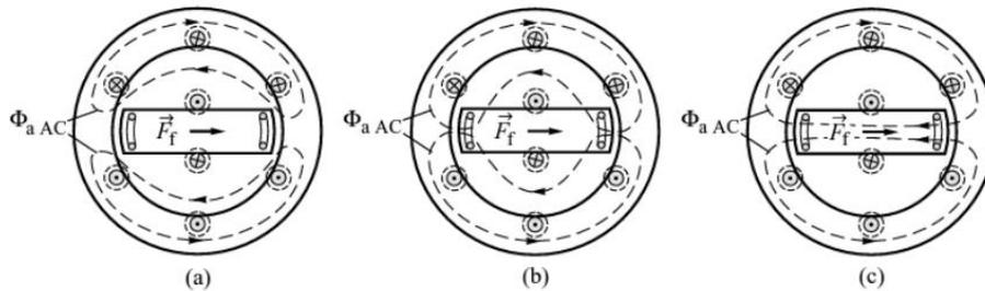
Figure 11 a) Sub-transient flux, b) Transient flux, c) Steady-state flux (d-axis) [6]
