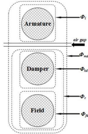
Figure 8 Magnetic fluxes illustration [4]
