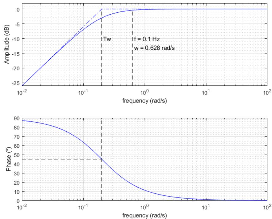
Figure 46 High-pass (washout) filter
