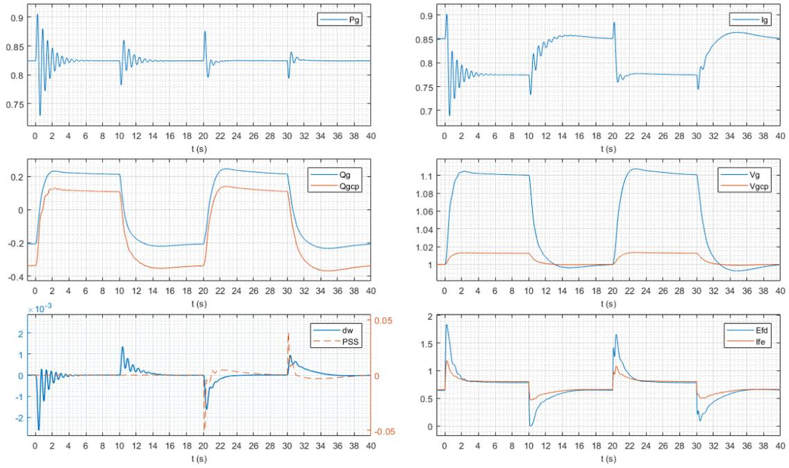
Figure 55 Step in the reference voltage 10% (time < 20 s – with PSS, time > 20 s – without PSS)
