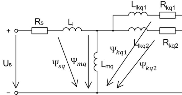
Figure 10 q-axis equivalent diagram with the fluxes
