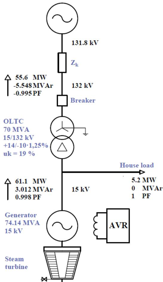
Figure 44 Load flow diagram of Power Generating Unit
