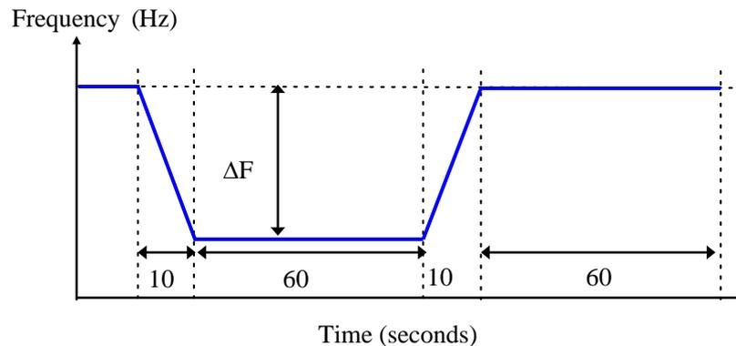
Figure 71 LFSM-U curve [1]
