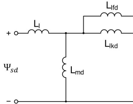
Figure 13 Equivalent circuit for  $L_d''$
