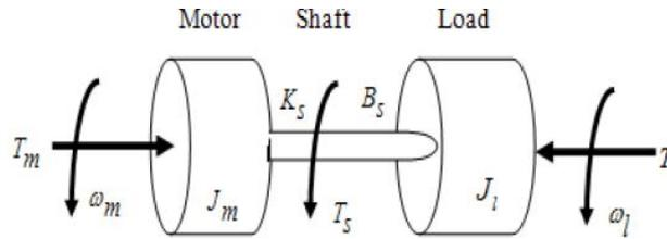
Figure 37 Rotating mass connected through shaft [10]
