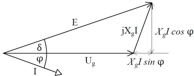
Figure 50 Load angle
