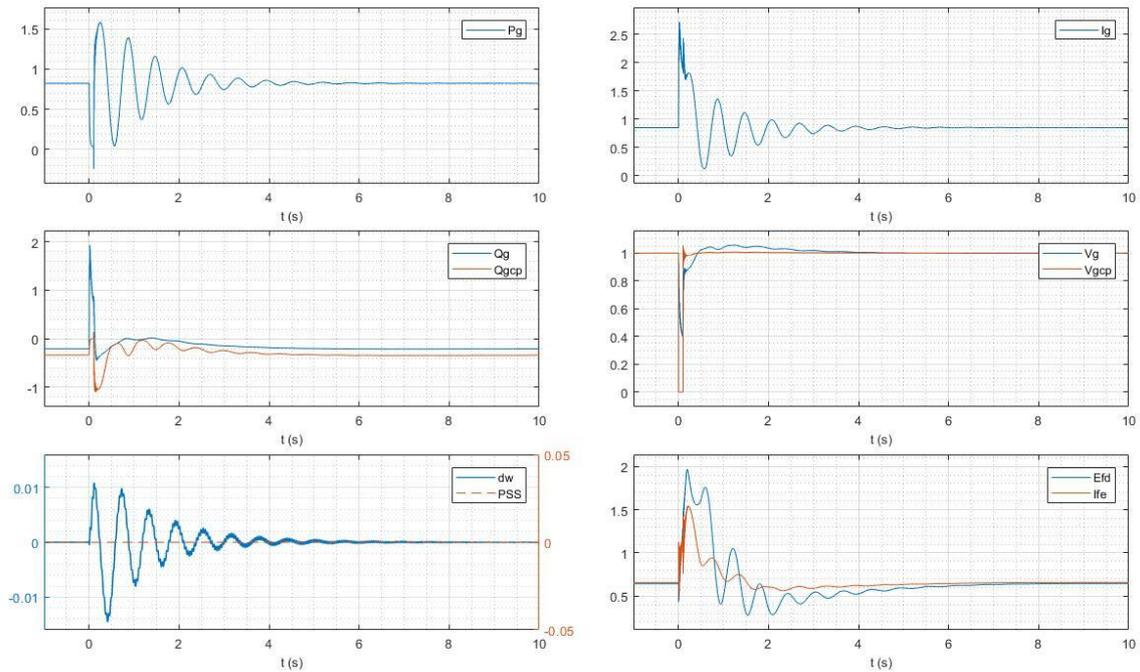
Figure 57 Voltage dip of 100 ms at HV terminal of the transformer - PSS OFF
