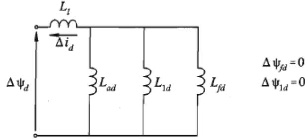
Figure 12 Flux deviation in the equivalent circuit [3]
