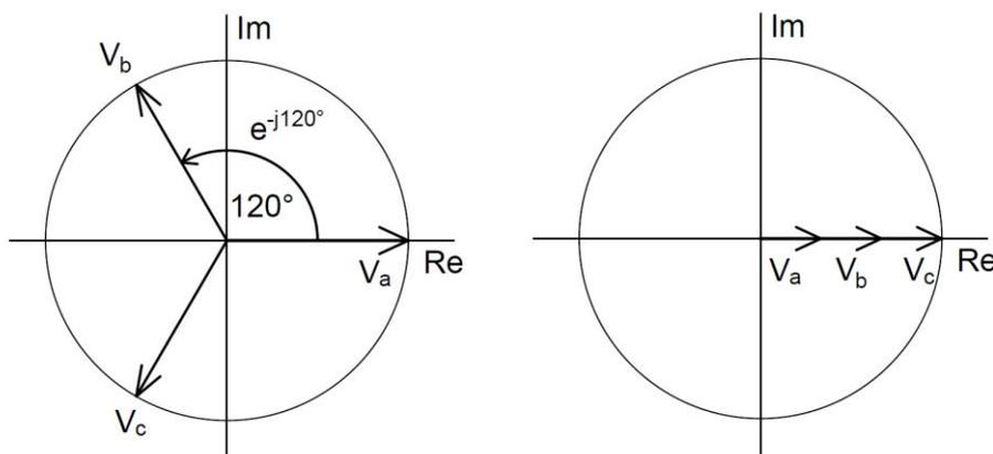
Figure 24 a) Phasors b) Positive sequence illustration
