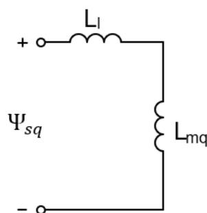
Figure 18 Equivalent circuit for \$L\_q\$
