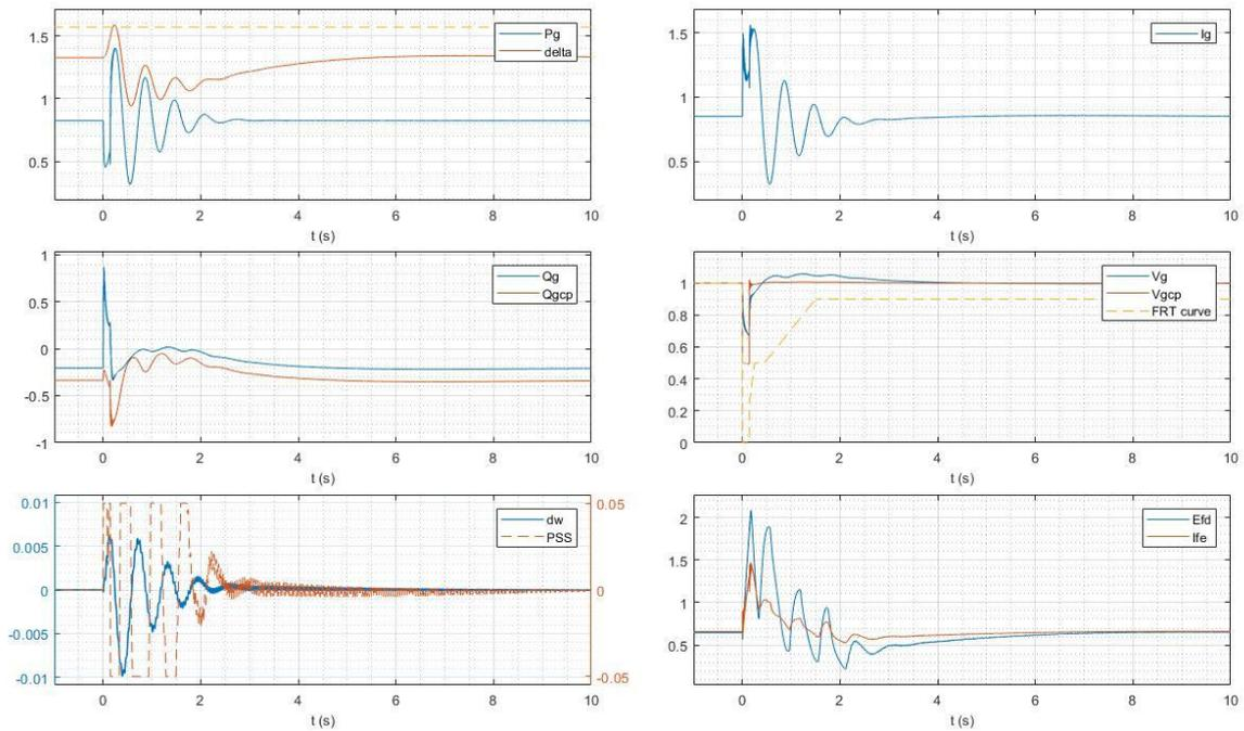
Figure 68 Ph-Ph short circuit at transformer terminals for 140 ms
