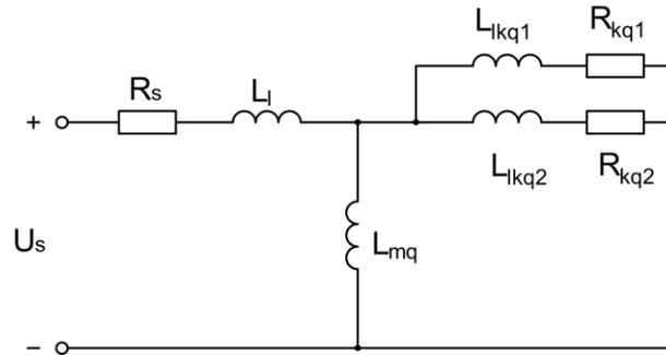
Figure 7 q-axis equivalent diagram
