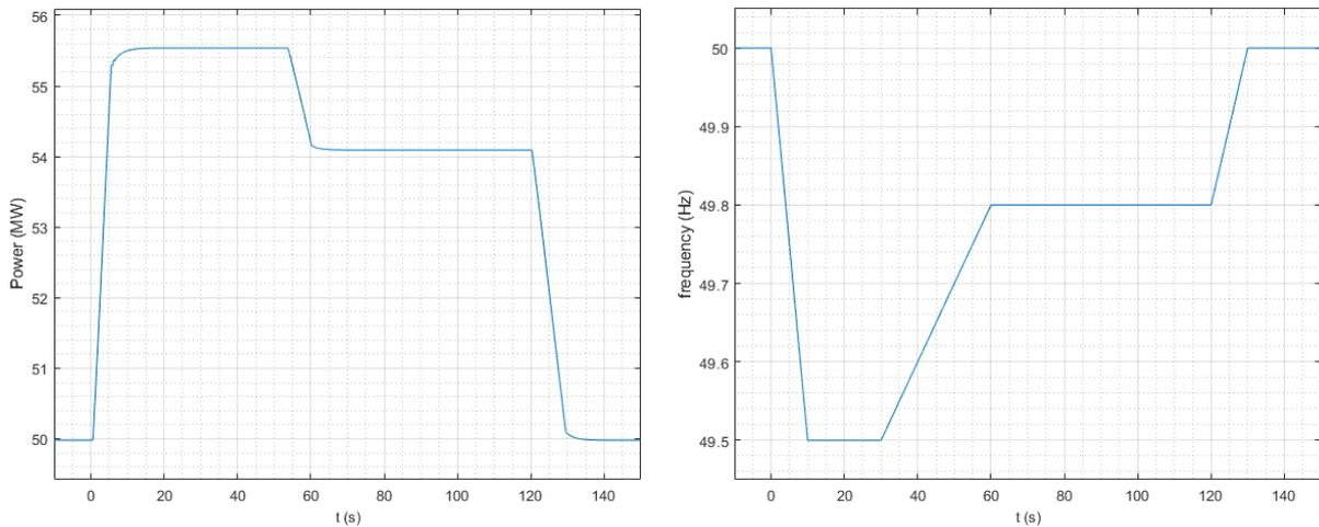
Figure 73 Frequency injection and power reaction
