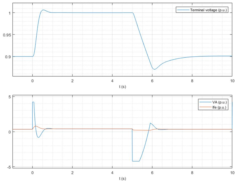
Figure 75 Reference voltage step from 90 % to 100%
