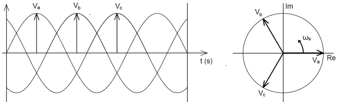
Figure 2 Harmonic waveforms of phases transform into phasors
