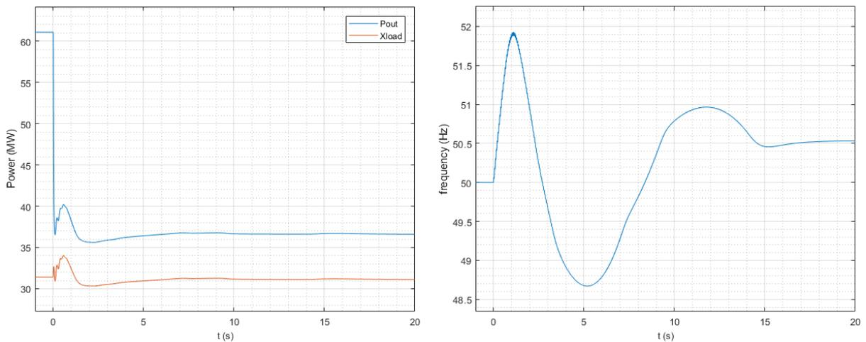
Figure 70 Grid cut-off with minimum possible connected load, LFSM and FSM
