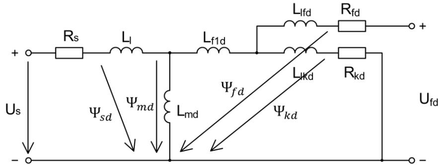
Figure 9 d-axis equivalent diagram with the fluxes
