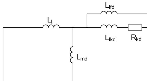
Figure 20 Simplified short-circuited diagram for the sub-transient interval ( $T_d''$ )
