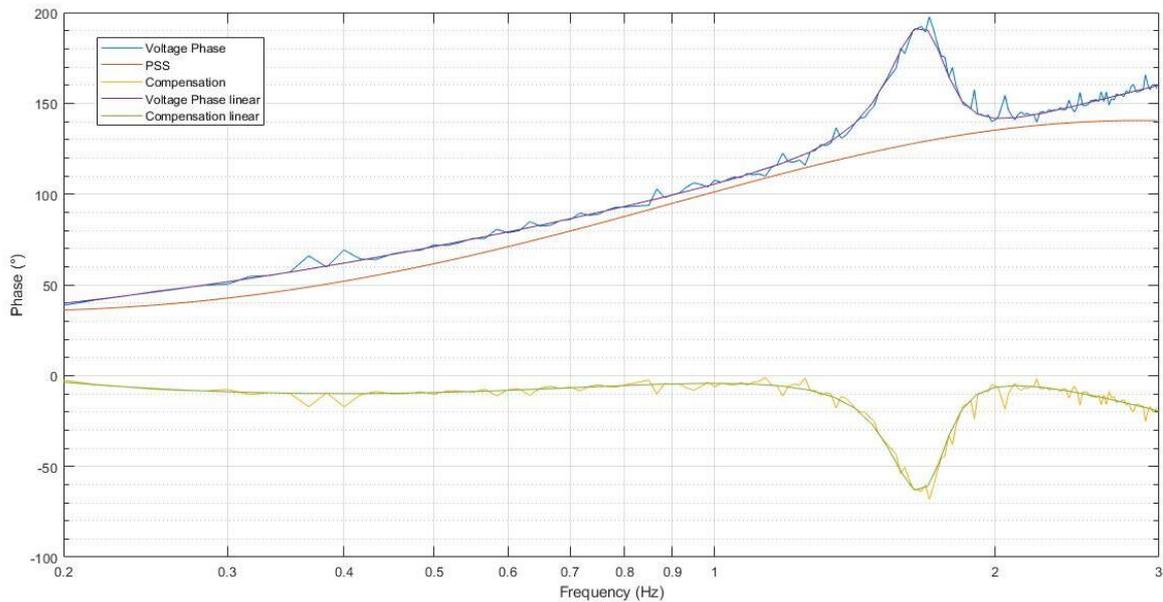
Figure 52 Voltage response and phase compensation by PSS
