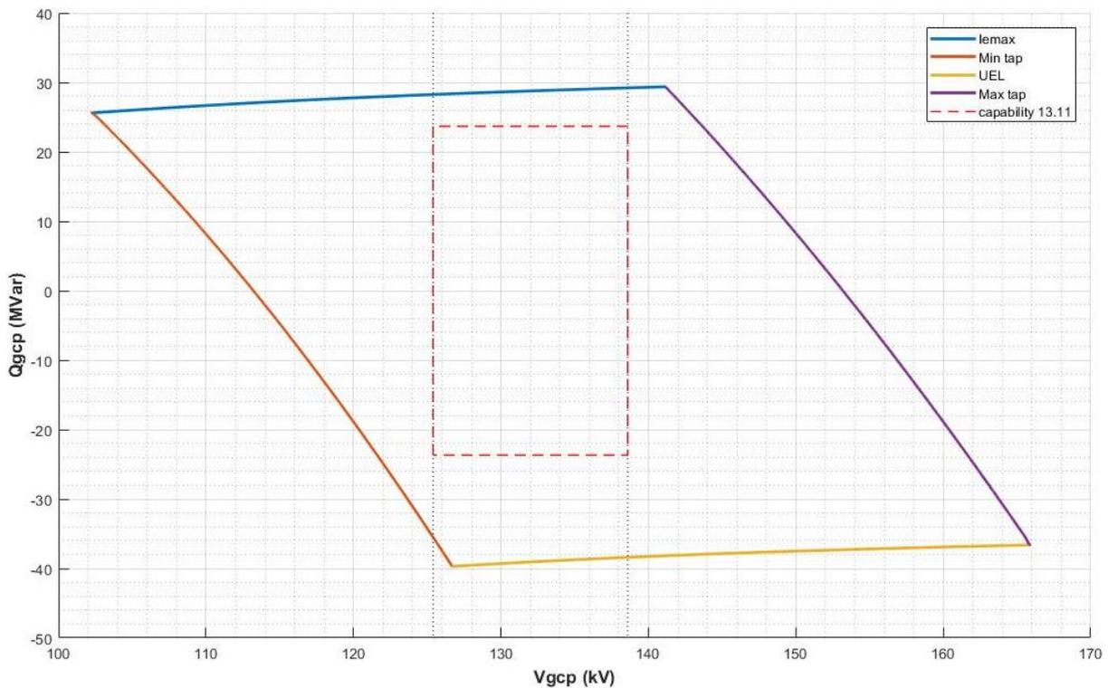
Figure 63 UQ capability diagram complying with specified conditions (i) and (ii)
