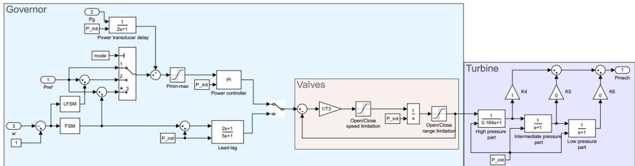
Figure 30 Simplified turbine model
