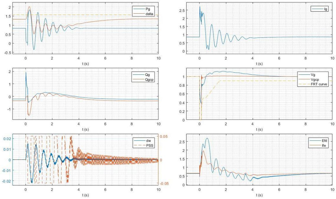
Figure 65 3-Ph short circuit at transformer terminals for 140 ms
