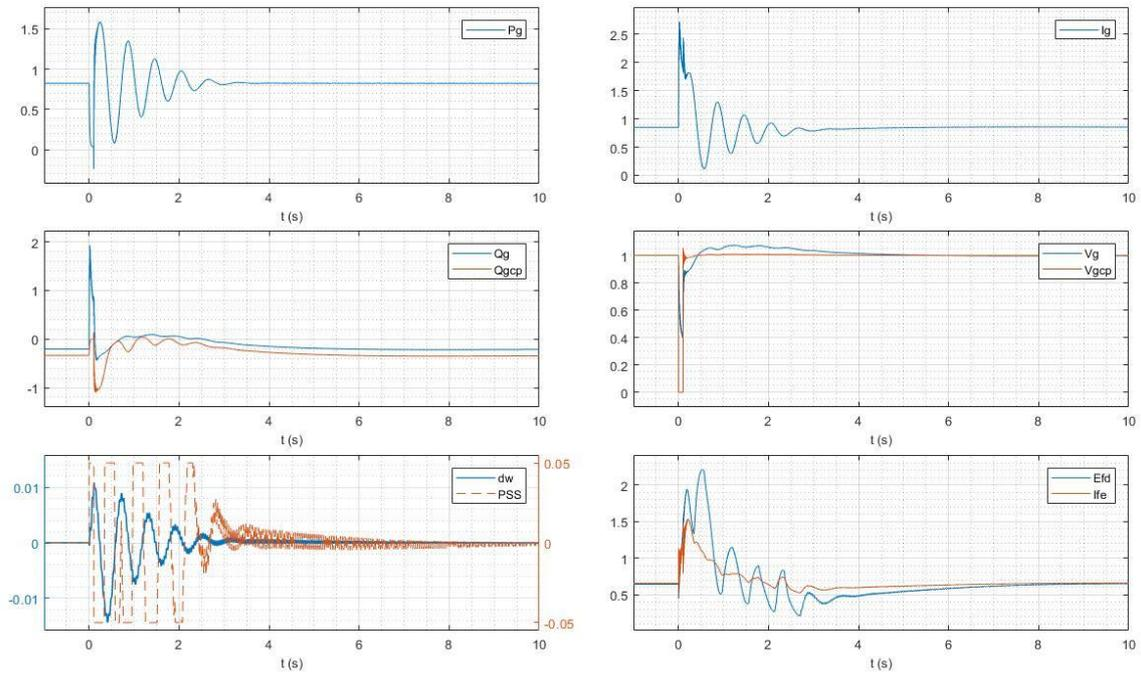
Figure 56 Voltage dip of 100 ms at HV terminal of the transformer - PSS ON
