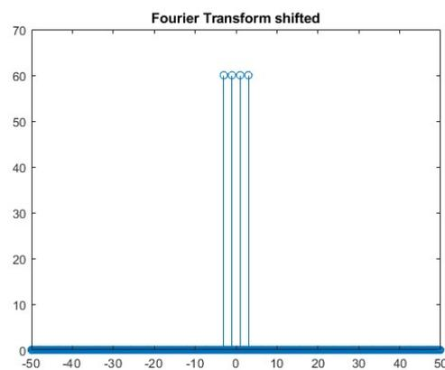
Figure 49 Visualization of the mirrored frequency spectrum
