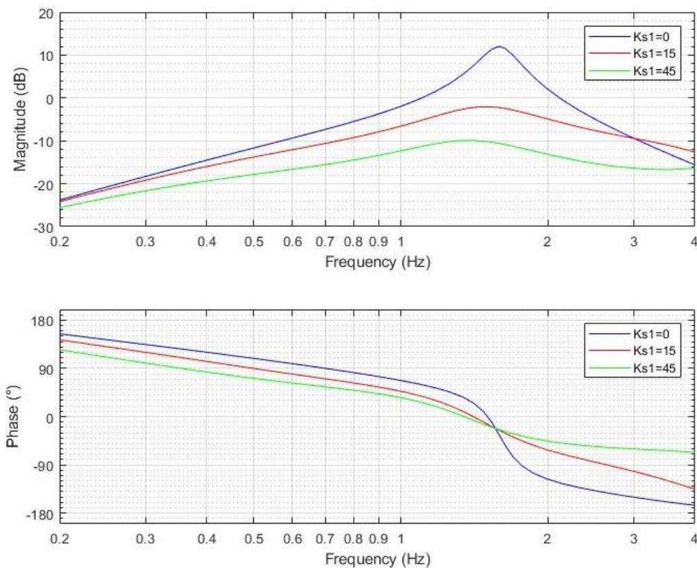
Figure 61 Bode plot  $P_m/V_{ref}$  in closed loop
