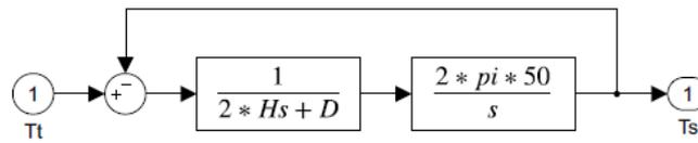
Figure 39 Implementation of mass equation in per unit
