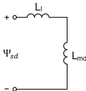
Figure 15 Equivalent circuit for  $L_d$
