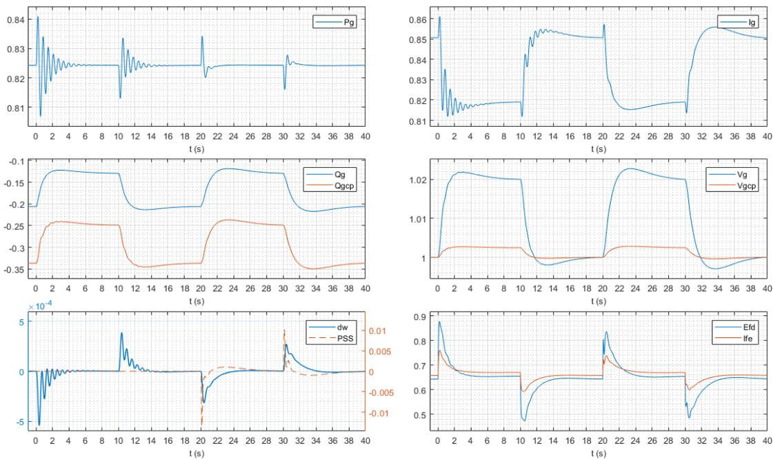
Figure 54 Step in the reference voltage 2% (time < 20 s – without PSS, time > 20 s – with PSS)
