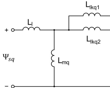
Figure 16 Equivalent circuit for \$L\_{q''}\$
