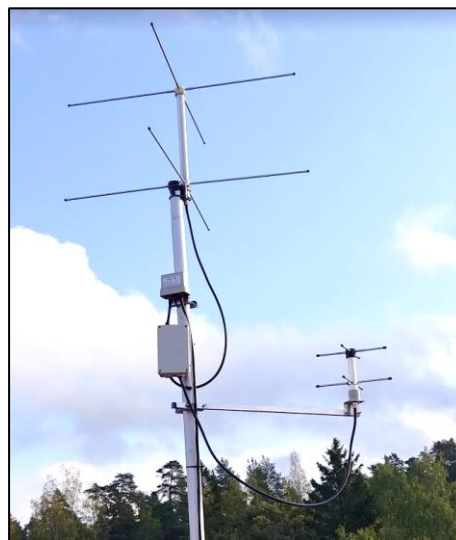
Figure 14. An illustrative picture showing how simple the omnidirectional antenna system for SDR-based GS from the network of SatNOGS [19].
