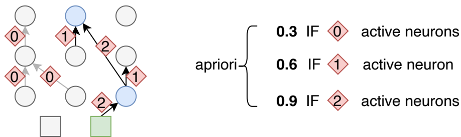
Fig. 4.19 The prior probability of activating an agents is based on its current surroundings.
