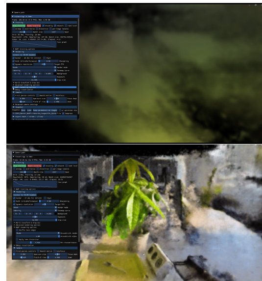
Figure 1: Training of a neural radiance field using the Instant-NGP algorithm, displayed in the Instant-NGP GUI [MESK22]. Rendering at initialization (top) and after 20 seconds of training (bottom). The object was captured from a 180-degree perspective, utilizing 145 images for training.
